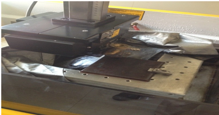
Figure 4.6 Photographic view of workpiece fixed on machining table
