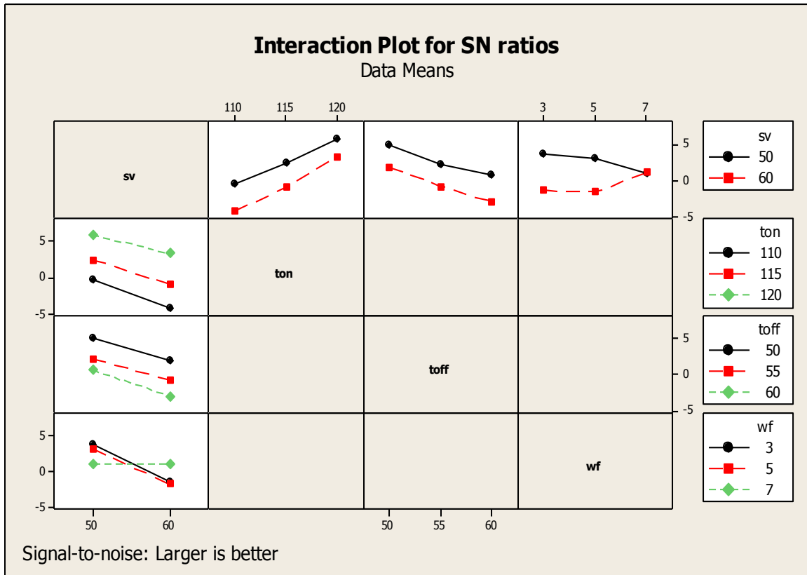
Figure 5.4 Effect of process parameter Interactions on MRR (Mean Data)
