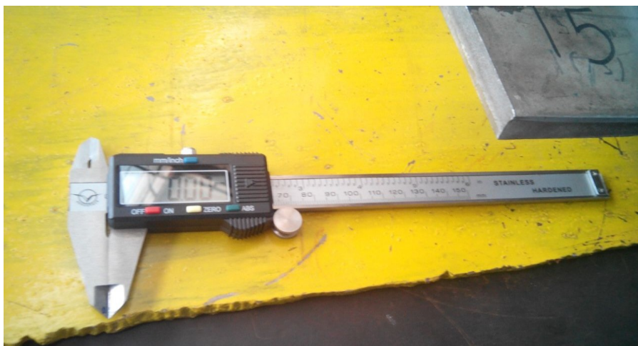
Figure 4.11 Photographic view of digital vernier calliper
