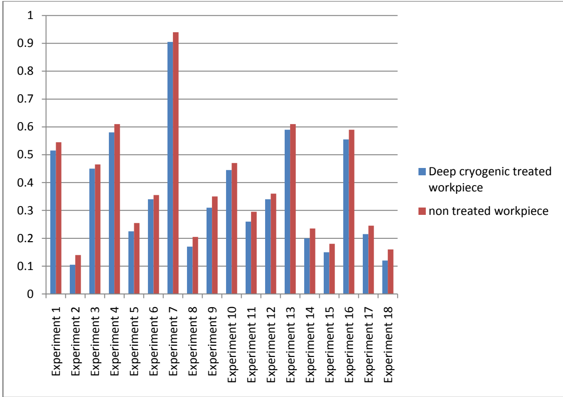
Figure 6.3 Bar graph for comparison of percentage of dimensional deviation
