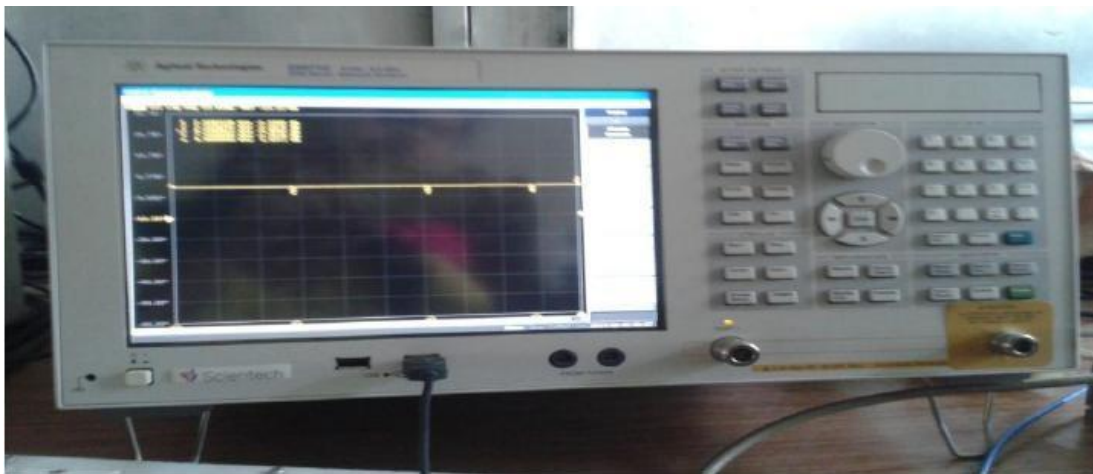
Figure 8.2 Vector network analyzer for testing
