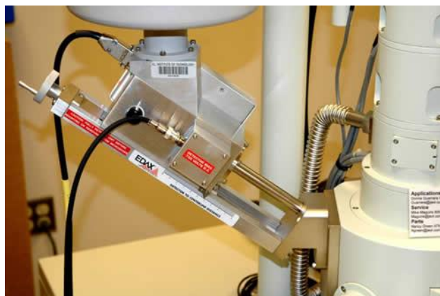
Figure 2.13 Pictorial view of EDAX attached to SEM [104]
