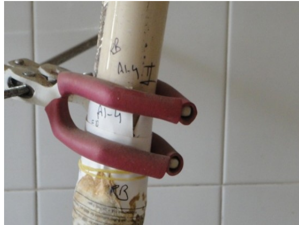
Fig. 4.6 Assembly of microbial sand column
