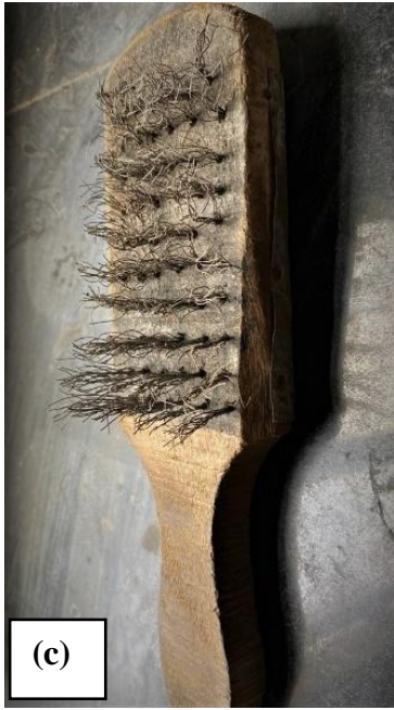
Fig. 3.26 Various stages of durability test; (a) wetting (b) drying (c) wired brush (d) specimen with the brush.
