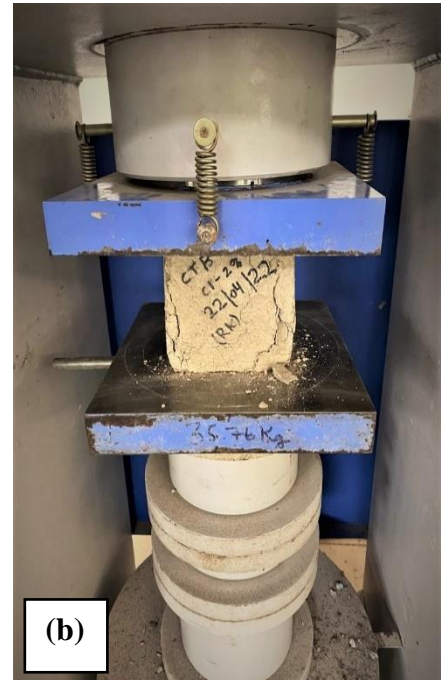
Fig. 3.25 Test setup for (a) Unconfined compressive strength (b) Specimen failure.
