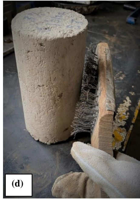
Fig. 3.26 Various stages of durability test; (a) wetting (b) drying (c) wired brush (d) specimen with the brush.
