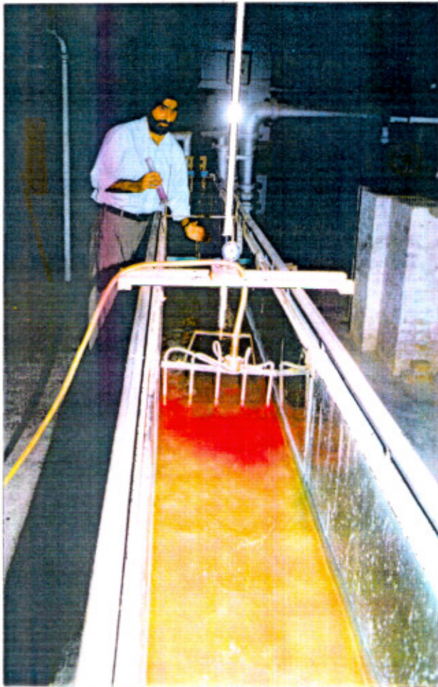
Fig. 4.8 A photographic view of tracer collecting sampler
