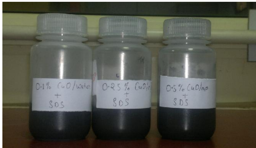
Fig. 4.2: Copper oxide distilled water based nanofluids (0.1 Vol. %, 0.25 Vol. % & 0.50 Vol. %)
