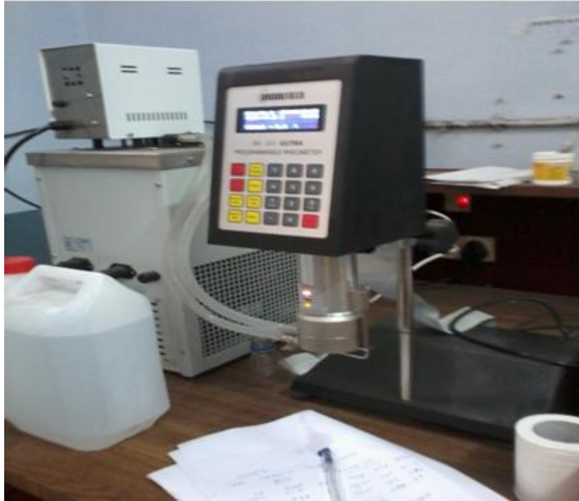
Fig. 4.18: Brookfield LVDV-III rheometer
