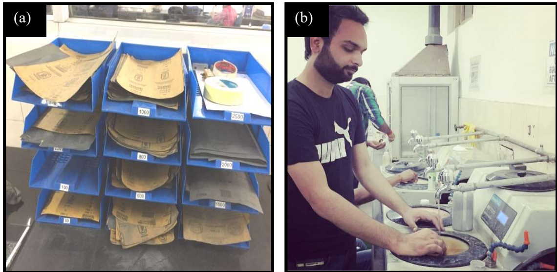
Figure 3.8: (a) Emery papers of average grit sizes of 80, 220, 320, 400, 800, 1000, 1200, 1500, and 2000, (b) Banipol Metco PMV018 used for polishing purposes.
