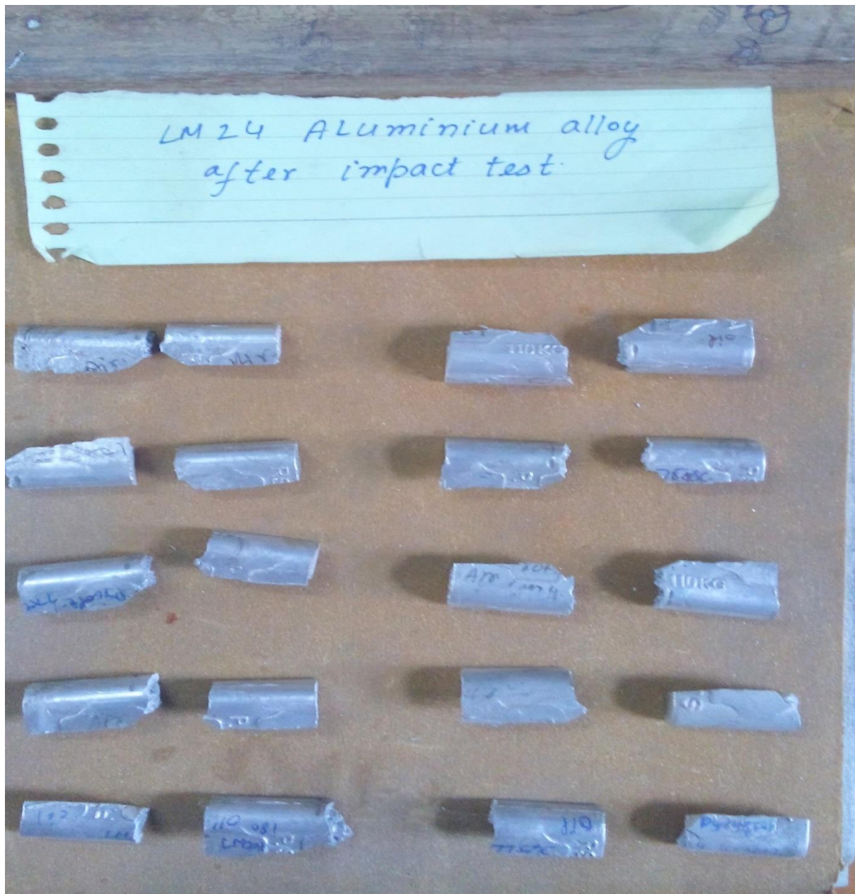
Fig.3.7 Material after impact test
