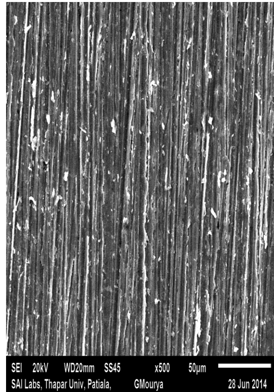
Figure 5.6 Microstructure of LM24, Pouring temp 725^{\circ} , injection pressure 190 \text{ kg/cm}^2 , Oil+ graphite coating, Air cooling
