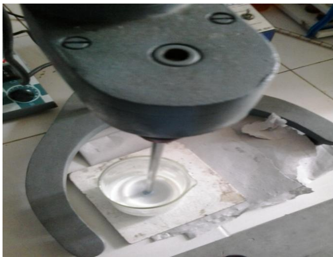
Fig. 3.1 Setup of Mechanical Stirrer
