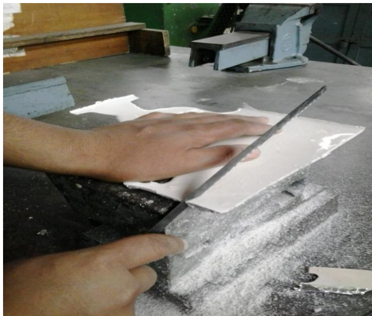
Fig. 3.3 Cutting of Specimen from sheet
