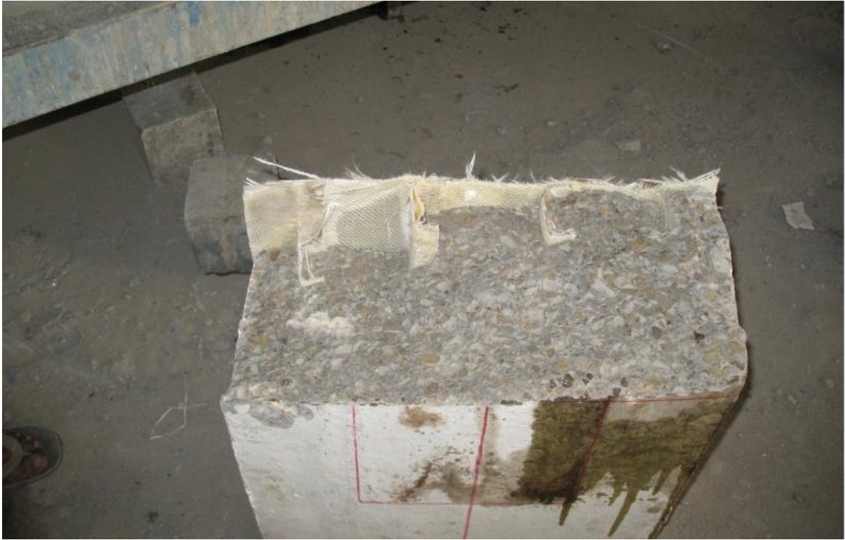
Fig.7.36 Breakage of form F11
