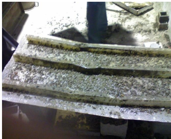
Fig 7.4 Buckling of channels in form D11
