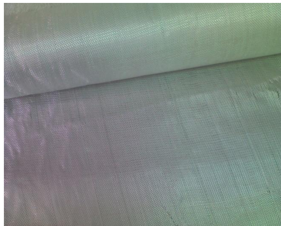
Fig.5.1. WRM 450 gsm GFRP used for making forms
