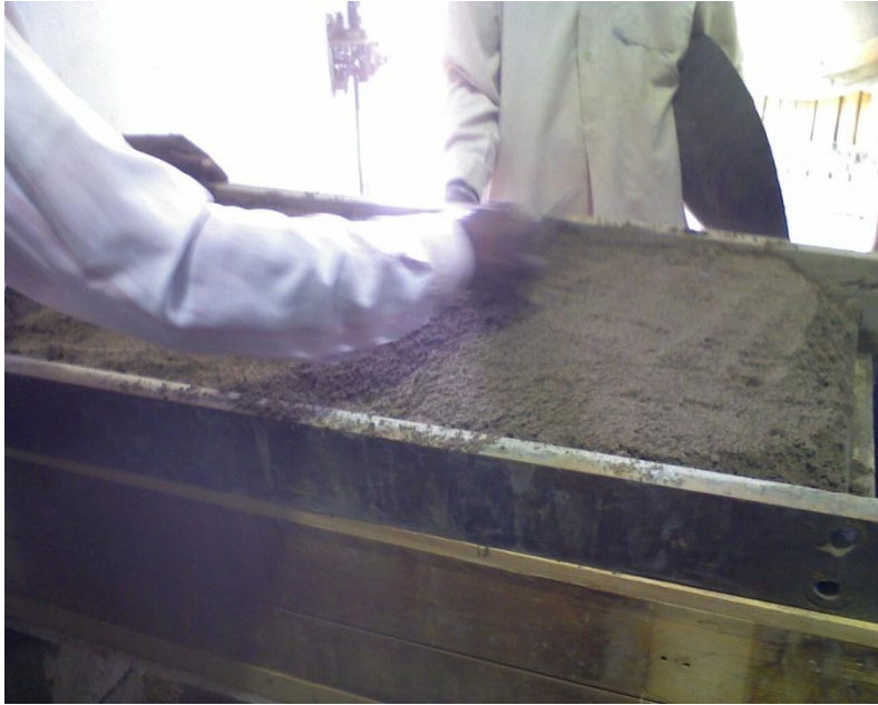
Fig 6.9b. Sand loading test on form F11
