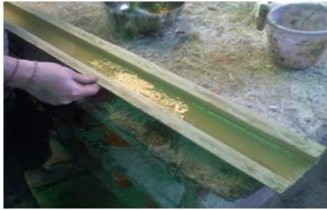
Fig.5.4. Applying gel coat on mould
