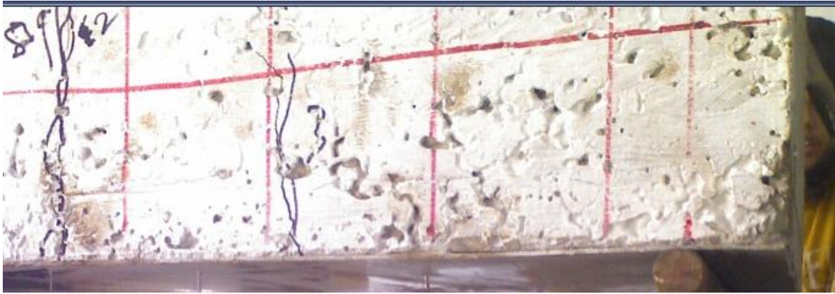
Fig.7.34 Slight delamination at load of 210kN
