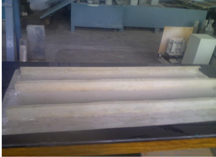
Fig.5.12. Prepared double layer base form with stiffener channels
