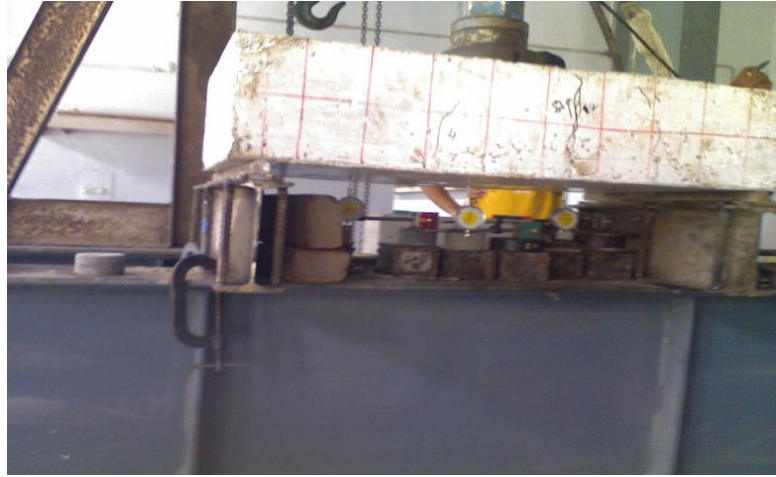
Fig.6.24 Test set up with stiffened supports
