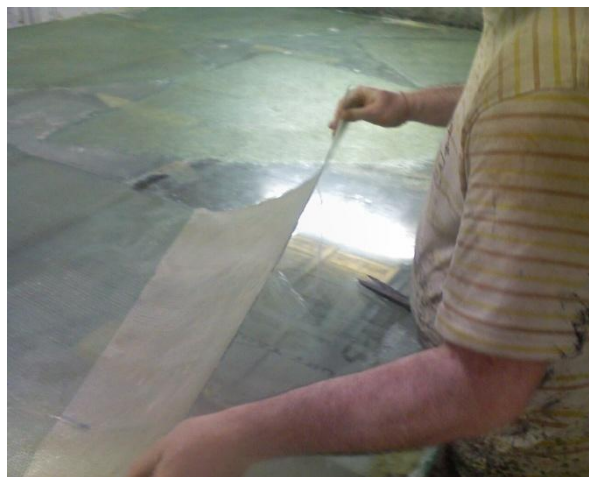
Fig.5.11. Removing single layer sheet from glass platform
