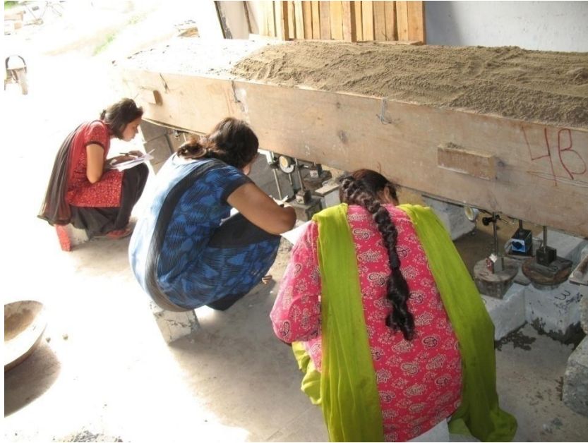
Fig.6.18. Sand test being carried out on form D13
