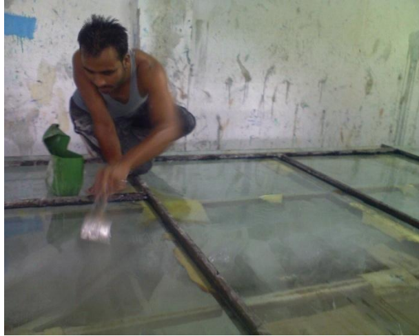
Fig.5.9. Applying initial resin layer on glass platform
