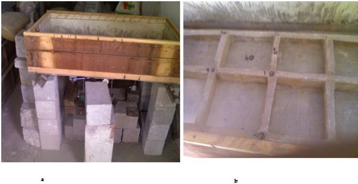
Fig6.7.a) Front view of the test set up b)Top view showing form within side forms
