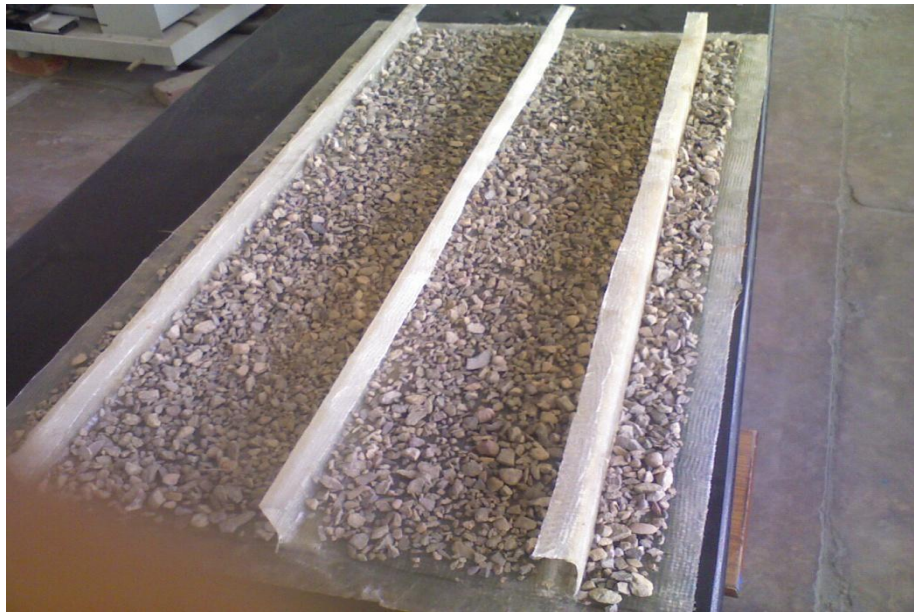
Fig.6.1. Form D11 coated with aggregates
