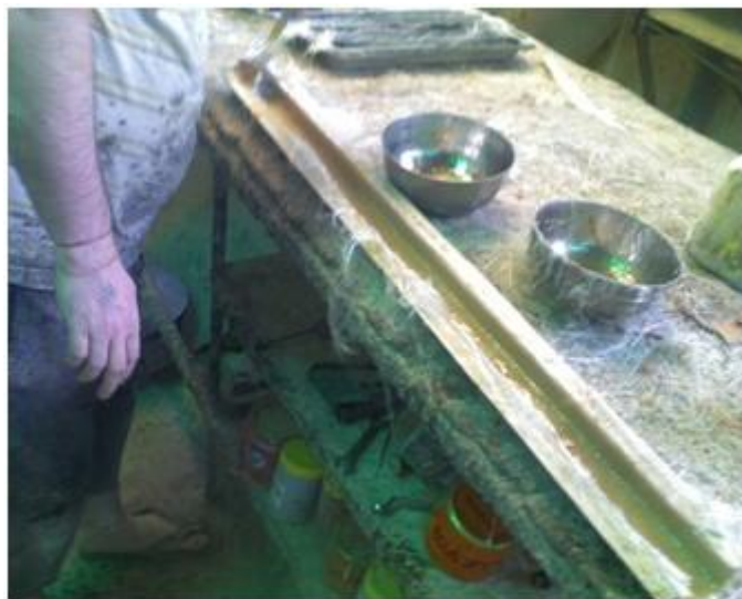
Fig.5.6. Applying resin coating on fiber sheet
