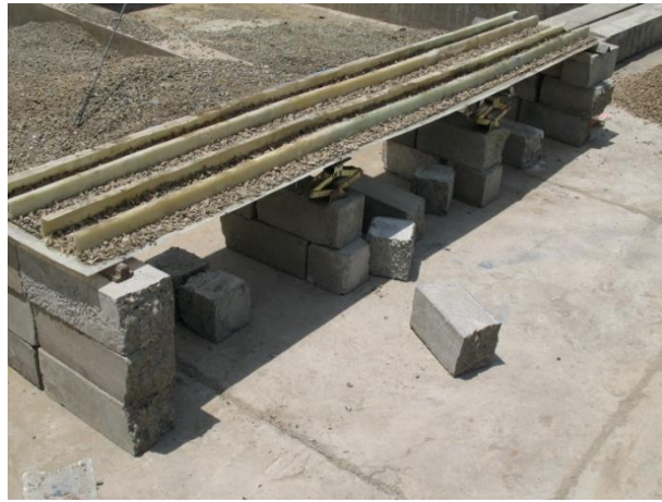
Fig.6.19. Use of car jacks during testing of form F23
