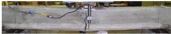
d) Flexural failure of specimen C1
