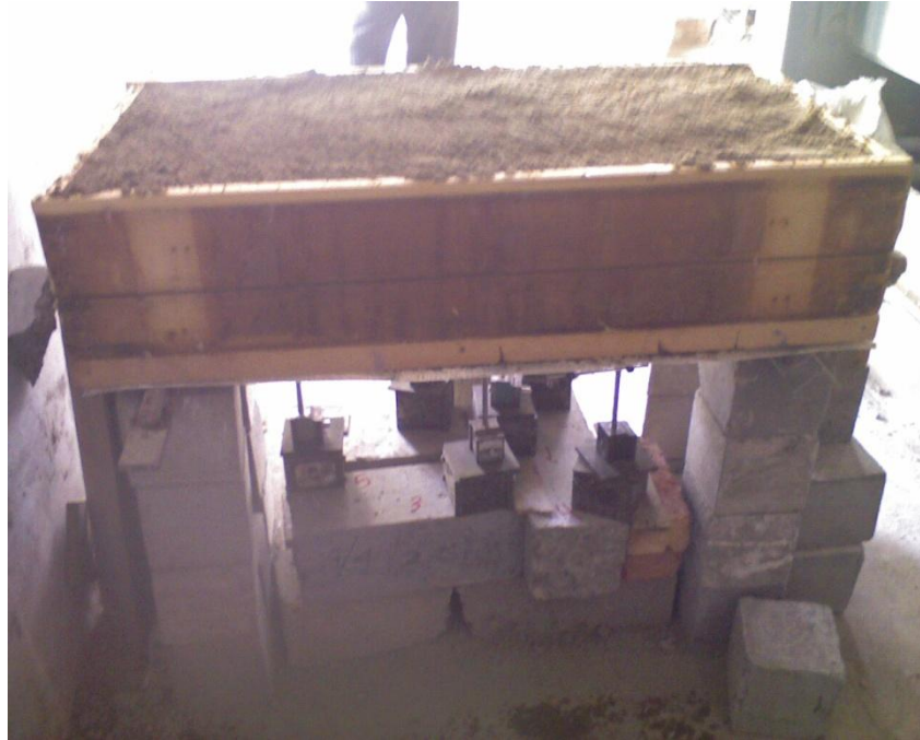
Fig.6.8. Sand loading test being done on form D21
