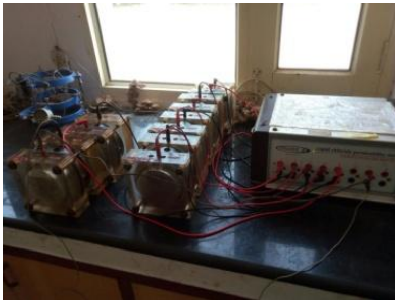
Fig. 3.2 RCPT test procedure setup
