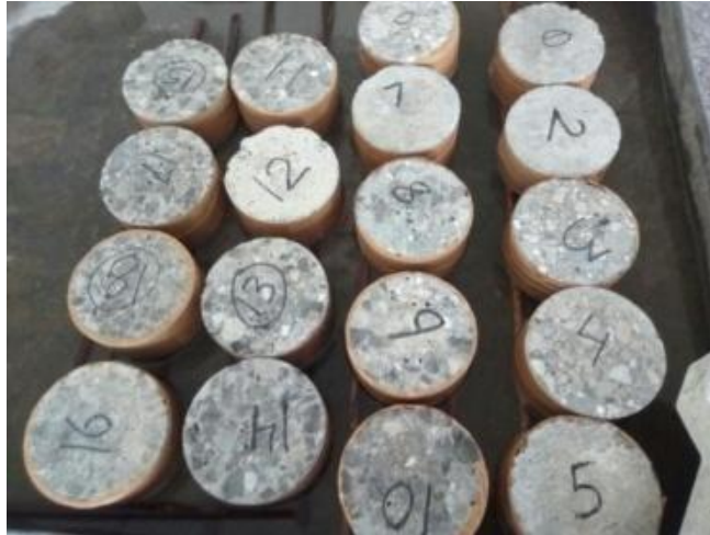
Fig. 3.3: Sorptivity test procedure setup
