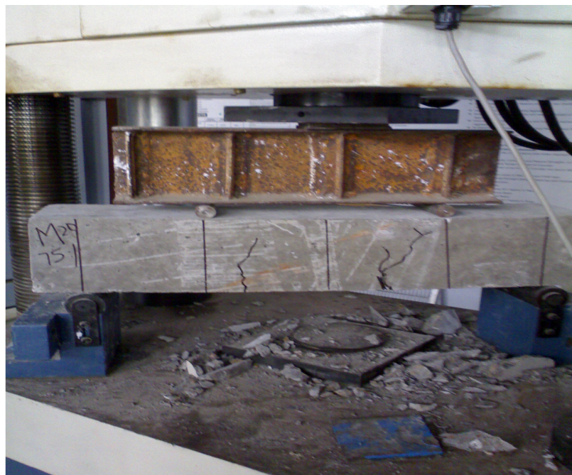
Plate -4.4: Stressing of M20 beam upto 75% of ultimate load
