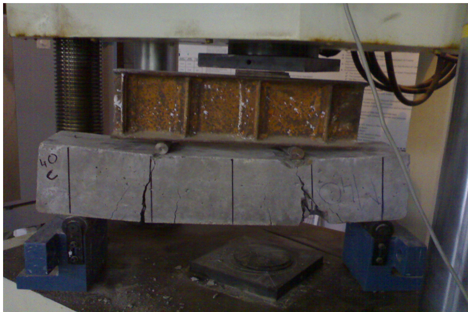
Plate – 4.2: Testing of M40 control beam
