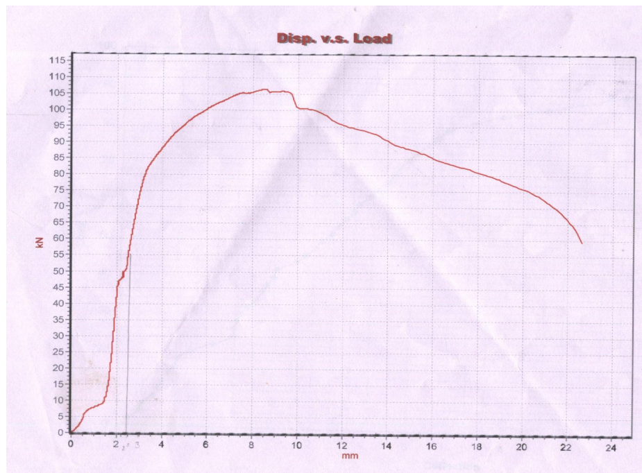
Figure .2 Load vs. Deflection curve for M20 control beam
