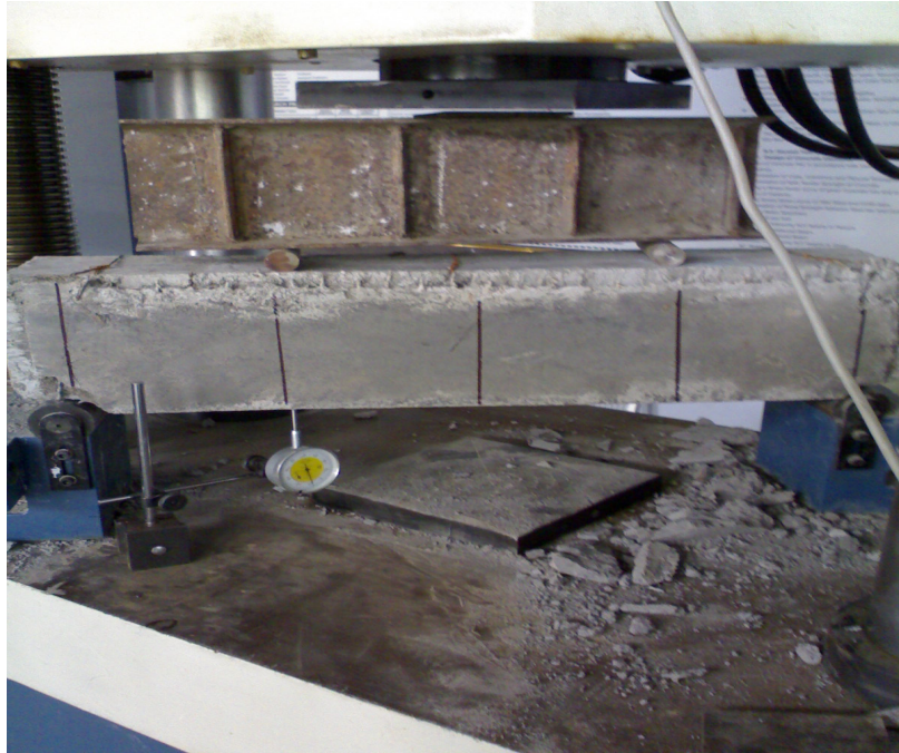
Plate -4.3 Testing of M40 retrofitted beam up to 50% of ultimate load.
