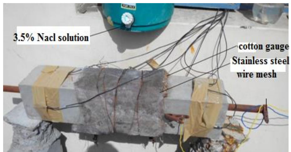
Fig.3.3: Test specimen with arrangement for induced corrosion
