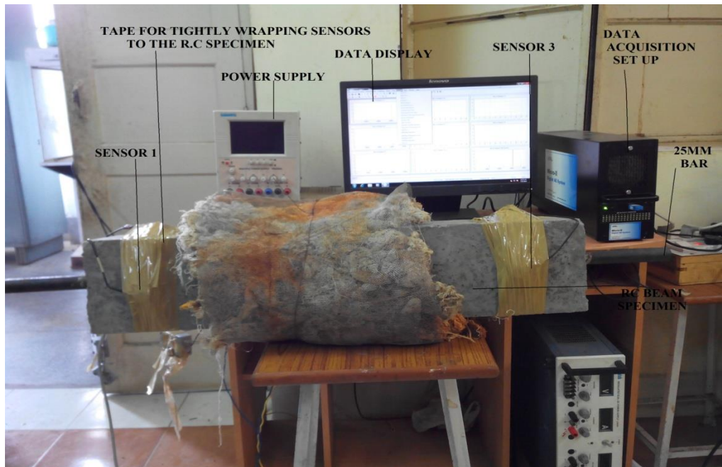
Fig.3.19: Experimental set up used in the study.
