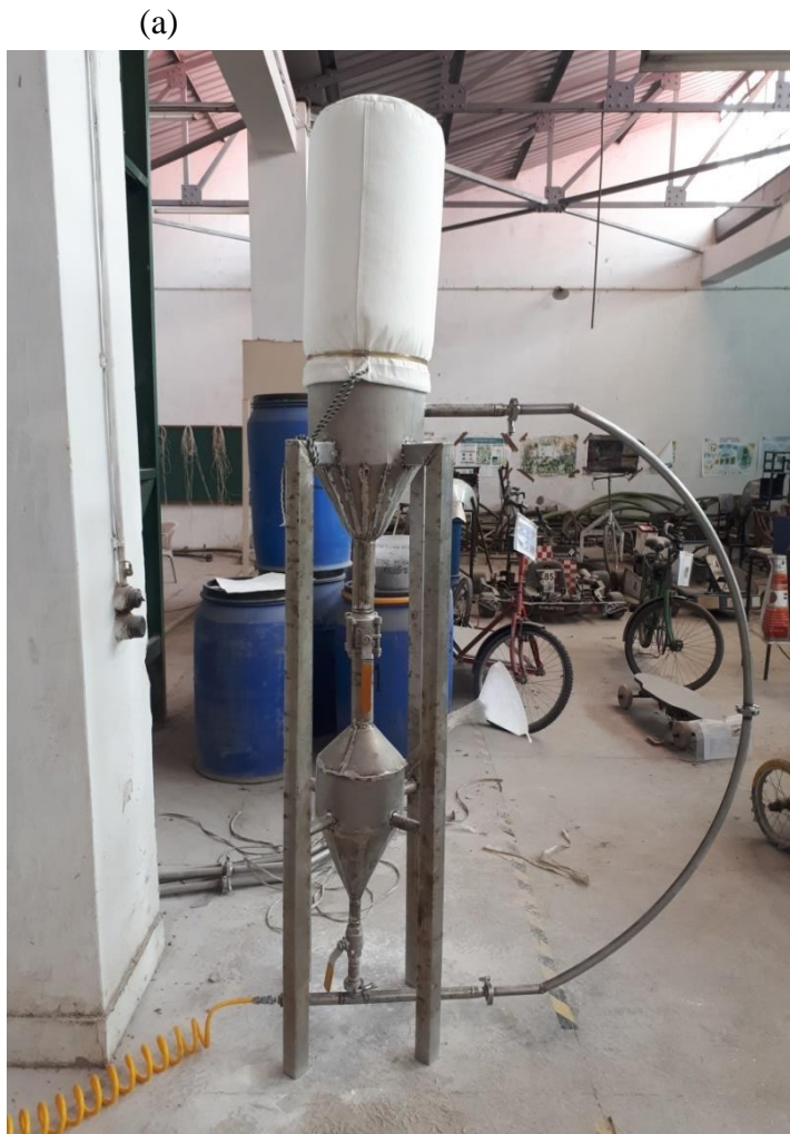
Figure 5.13. (a) Dry coating machine working with bend and bag filter attached to the upper hopper, (b) Connection from the air receiver to the suction line through yellow pipe
