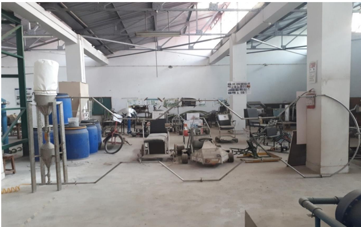
Figure 6.1. Dry coating machine functioning with the maximum conveying length of 8 sections and a bend connecting the upper and lower sections together with the hopper assembly and bag filter connected to the upper hopper
