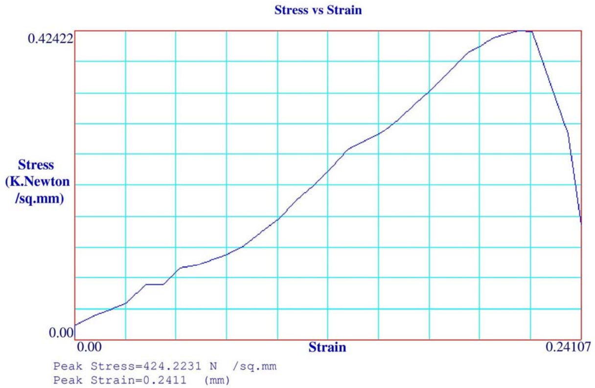
Fig 5.7: stress vs. strain curve for specimen which weld from flux 4
