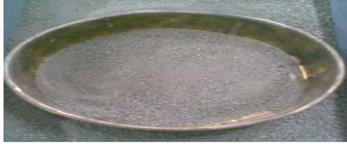
Fig 4.2: Test sieve (8 BS, 10 ASTM, 2 mm IS, 2057 microns)
