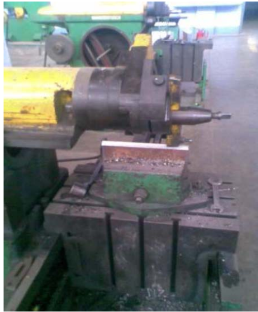
Fig 4.4: Making chamfer on corner of plate
