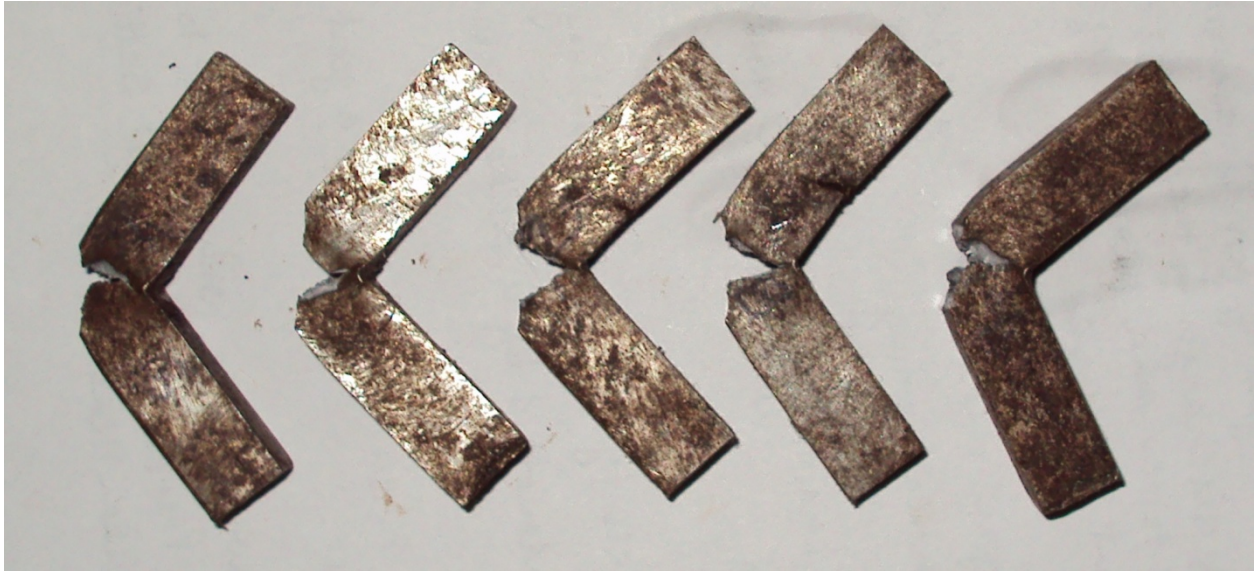
Fig 5.11: Specimen after impact test
