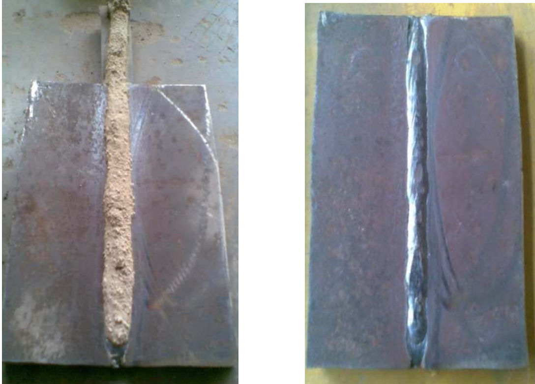
Fig 4.5: Joint of plates after welding
