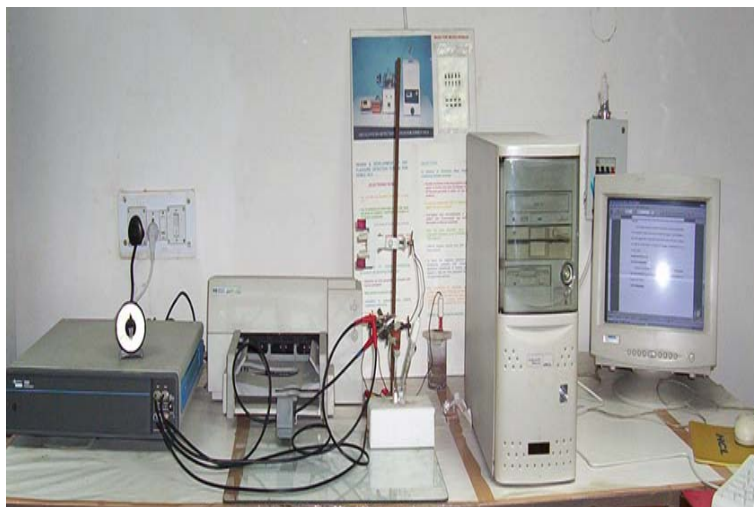
Fig 3.1: Electrochemical Interface (SOLARTRON Potentiostat 1285)
