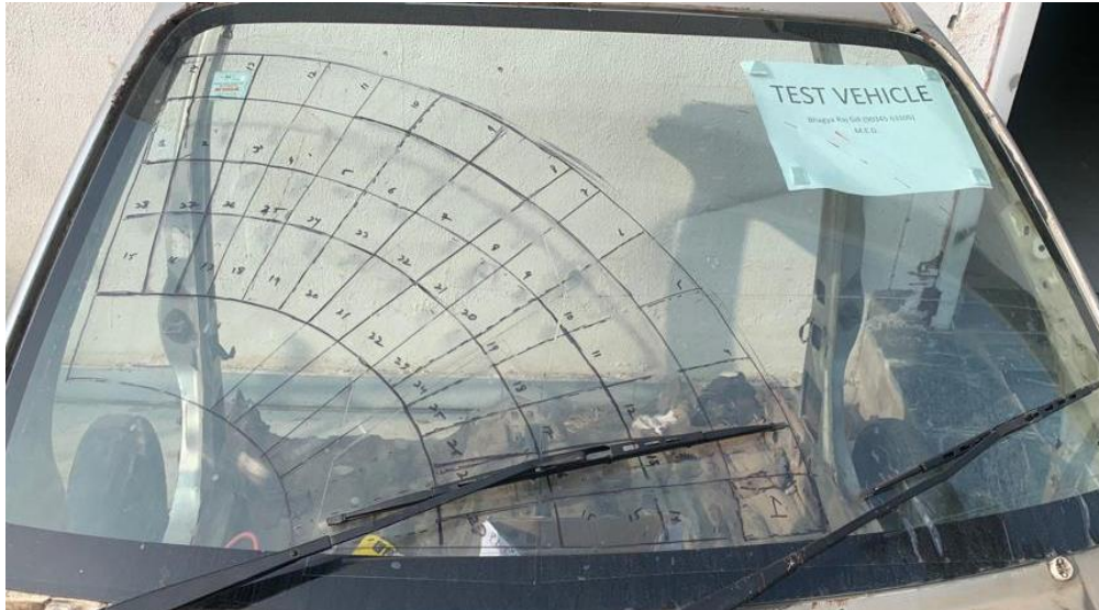
Fig. 4.4 Segmentation of Windshield
