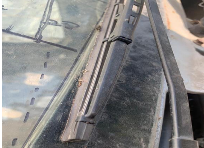
Fig. 1.3 Dust deposition on the wiper blades
