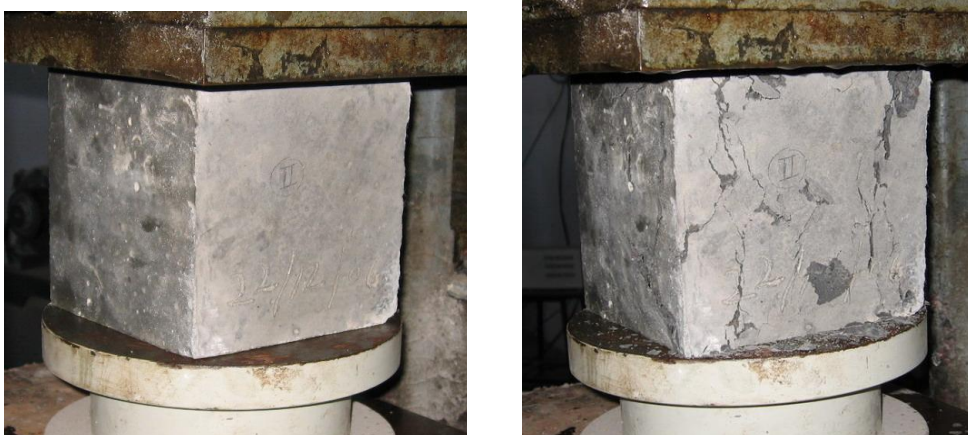
Figure 3.5 Compressive strength test of concrete cube specimens
