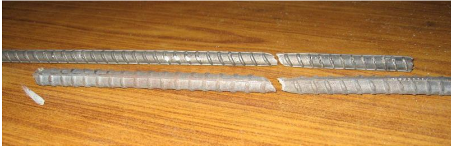
Figure 3.8 Failed reinforced steel bar samples
