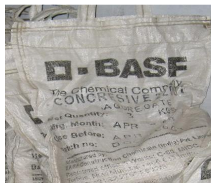
Figure 3.13 MBrace Putty: aggregate part C
