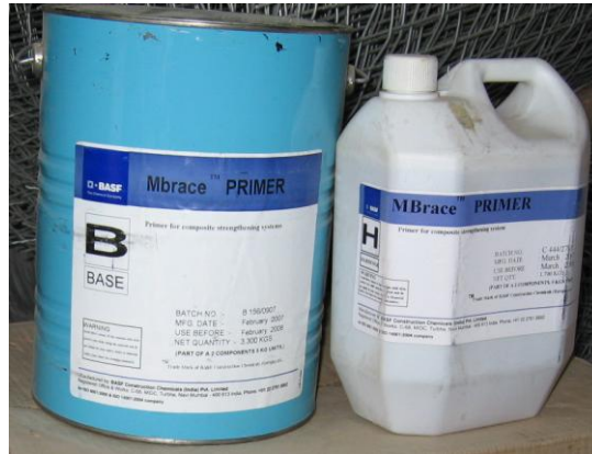
Figure 3.11 MBrace Primer: resin part A and hardener part B
