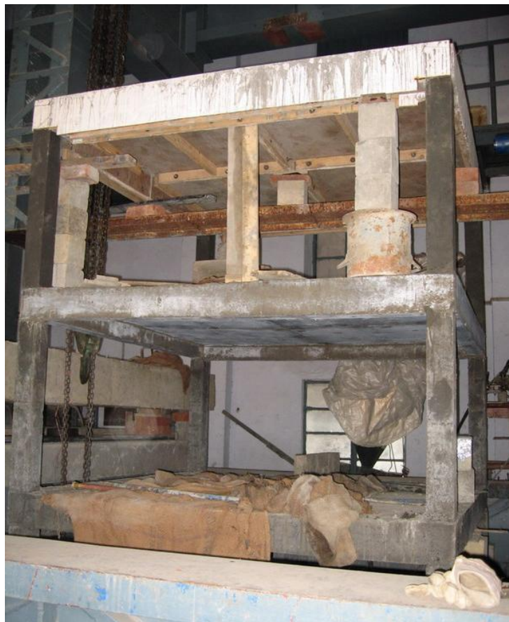
Figure 3.22 Curing specimens with wet sacks
