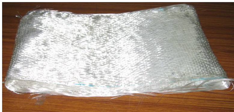
Figure 3.10 MBrace Fiber: glass fiber sheet (G sheet EU 900)
