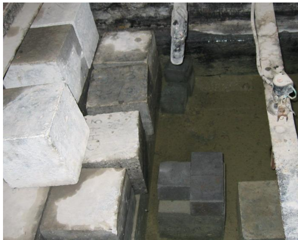
Figure 3.3 Concrete cube specimens in curing tank with temperature control
