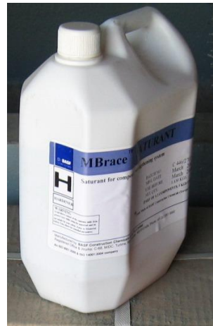
Figure 3.14 MBrace Saturant: resin part A and hardener part B
