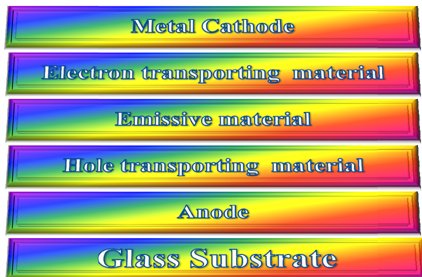
Figure 1.3: The structure of OLEDs
