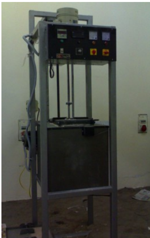
Figure 3.1: Electric Resistance Furnace used for Al foam production.
