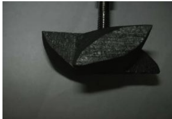
Figure 3.2: Graphite impeller used for melt stirring (Side view).
