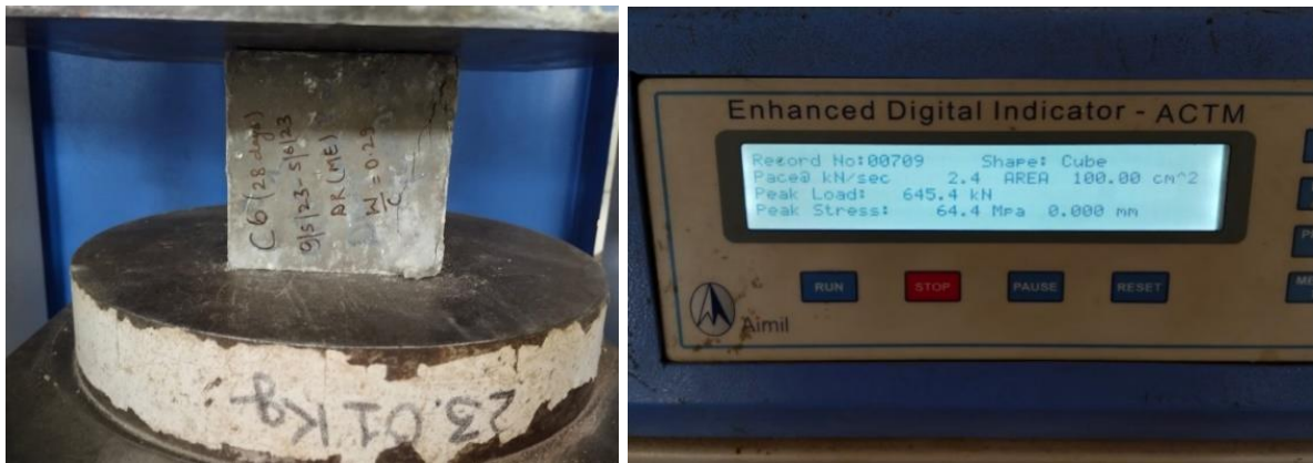
Figure 3.8 Testing of cubes and its strength after 28 days of Mix Design (M60)
