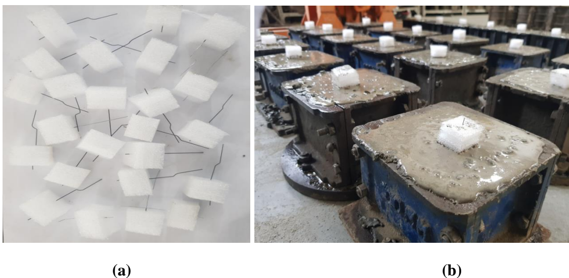
Figure 3.17 - (a) SMA marked for embedded length (b) Specimens for bond test
