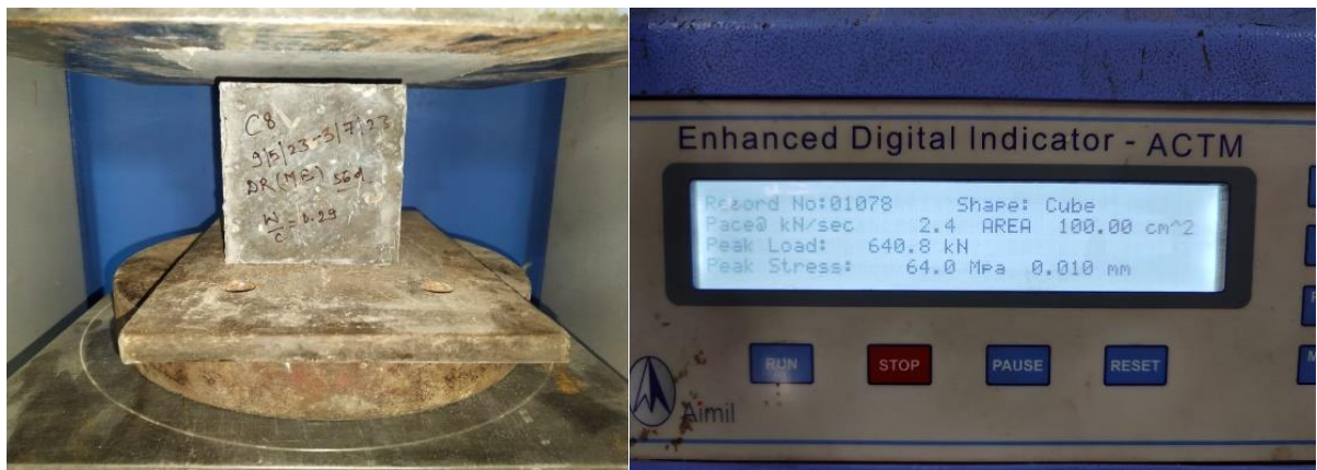
Figure 3.9 Testing of cubes and its strength after 56 days of Mix Design (M60)
