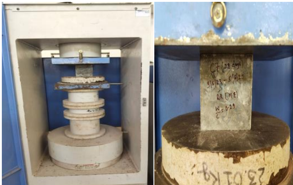
Figure 3.16 -Testing of specimen for compression in CTM
