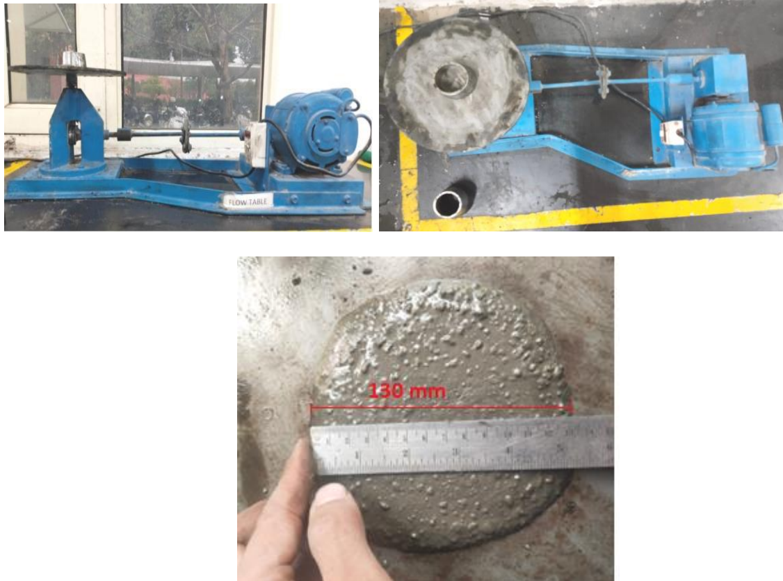
Figure 3.5 Flow table Instrument (a) Side view of flow table; (b) Top view of flow table; (c) Flow of concrete measurements
