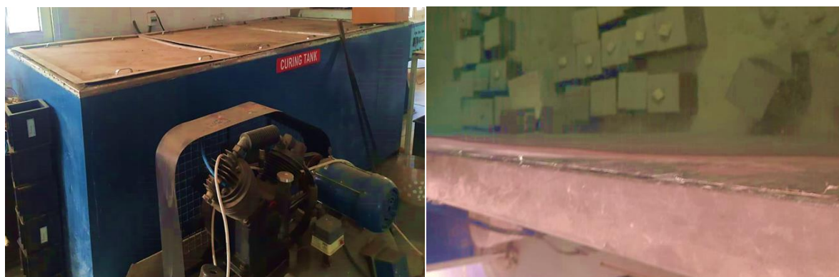
Figure 3.14 - Curing of samples in Curing tank
