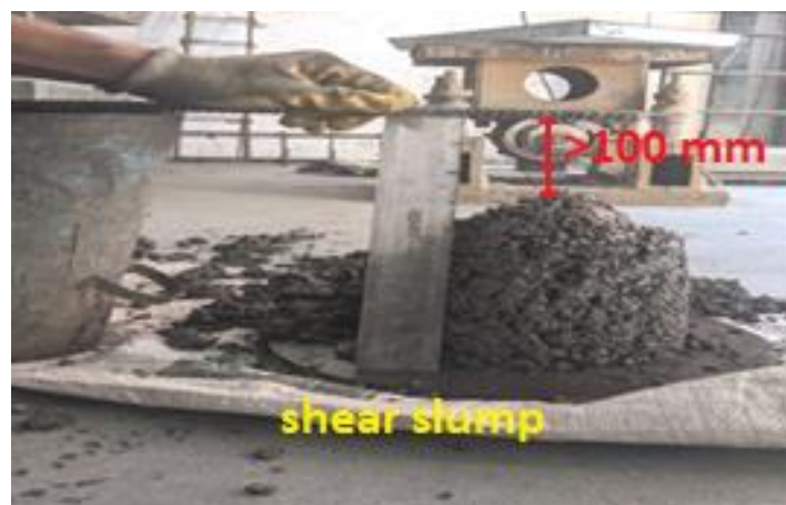
Figure 3.15 Slump measurement of concrete
