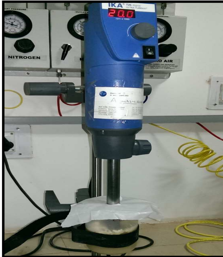
Fig. 3.1 Homogenizer system dispersing clay in the resin (Photo courtesy: Chemical Engineering Department, Thapar University, Patiala)
