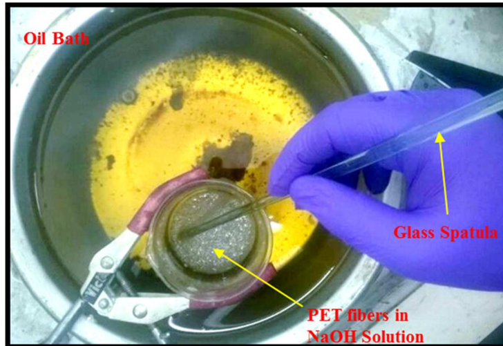
Fig. 3.14 Fibers dipped in NaOH solution in an oil bath
