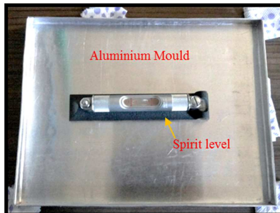
Fig. 3.10 Mould levelling using spirit level
