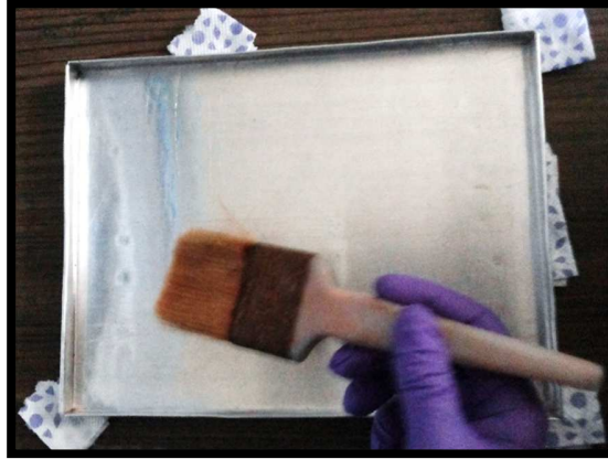
Fig. 3.11 Coating of mould with release agent
