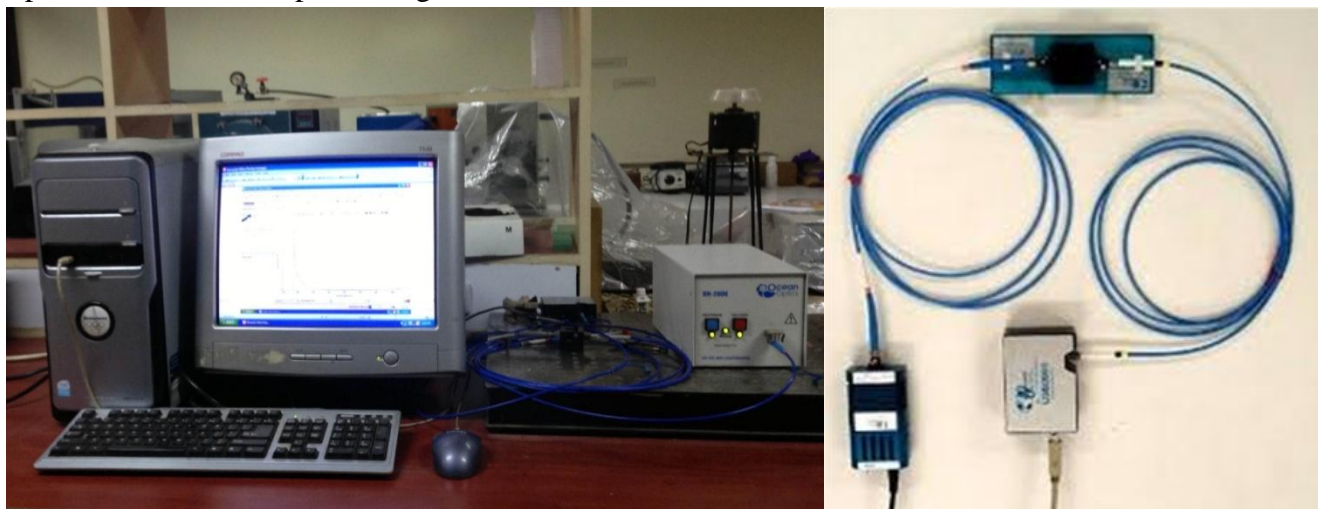
Figure 3.6: Experimental set of UV-visible spectrometer used
