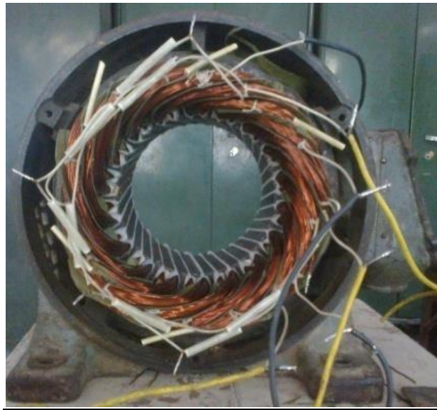
Fig. 2.2 Stator of Induction Motor
