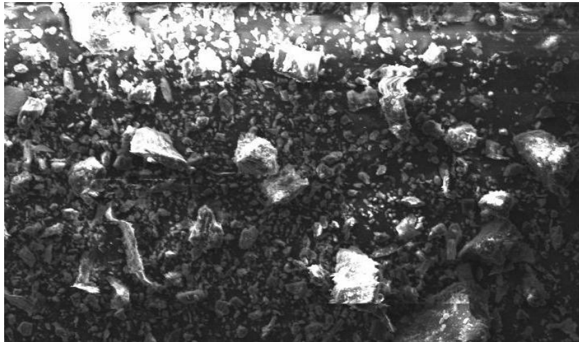
Fig. 3.5: SEM micrograph of S-IV coal sample ( d_{50}=110 \mu\text{m} )
