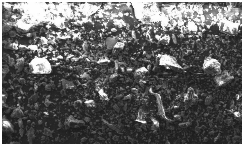
Fig. 3.6: SEM micrograph of S-V coal sample ( d_{50}=112 \mu\text{m} )
