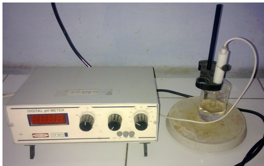
Fig. 3.7: Digital pH meter used for measuring slurry pH
