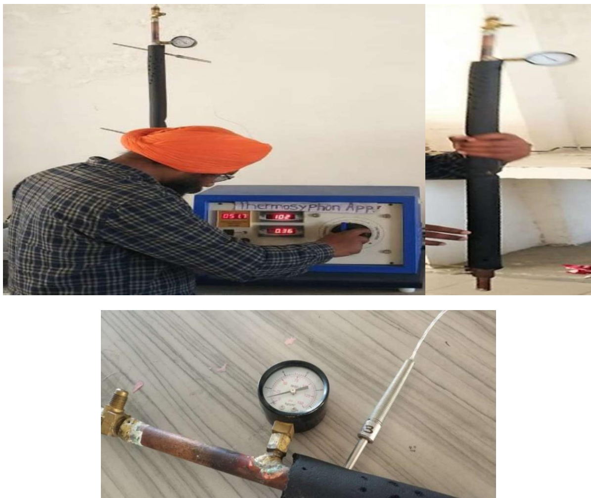
Figure: 5.1 Thermosyphon setup
