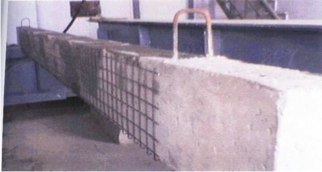
Plate 3.3: Beam with wire mesh at 0 degree
