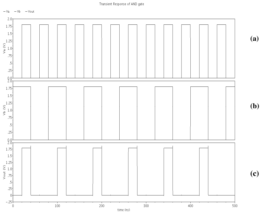
Figure 5.4 Simulation Results of Two-Input CMOS AND Gate
