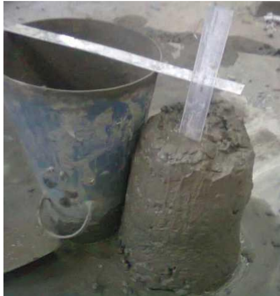
Figure 3.3: Experimental set up for measuring slump of fresh concrete
