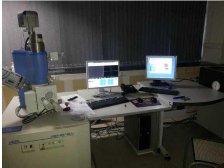
Figure 3.9: Experimental set up for scanning electron micrograph
