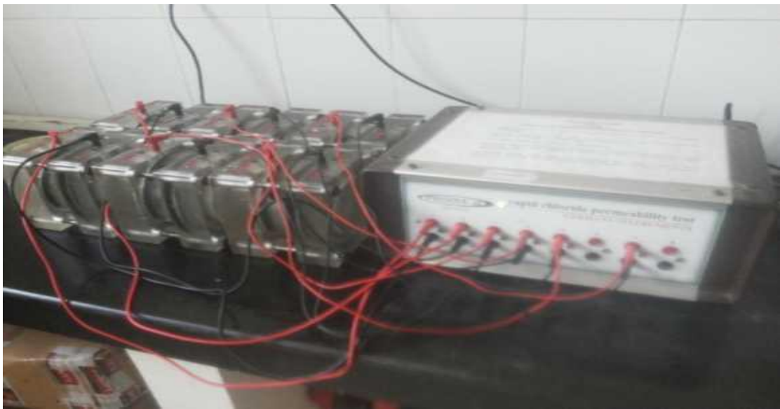
Figure 3.7: Experimental set up for measuring chloride ion penetration
