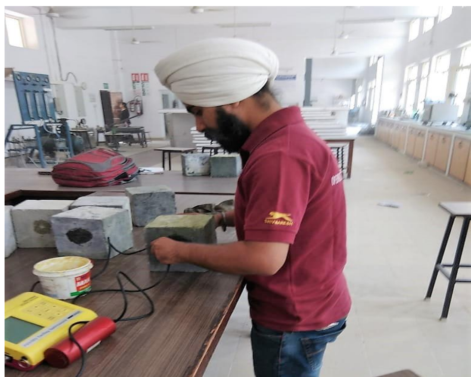
Figure 3.6: Testing of pulse velocity of concrete
