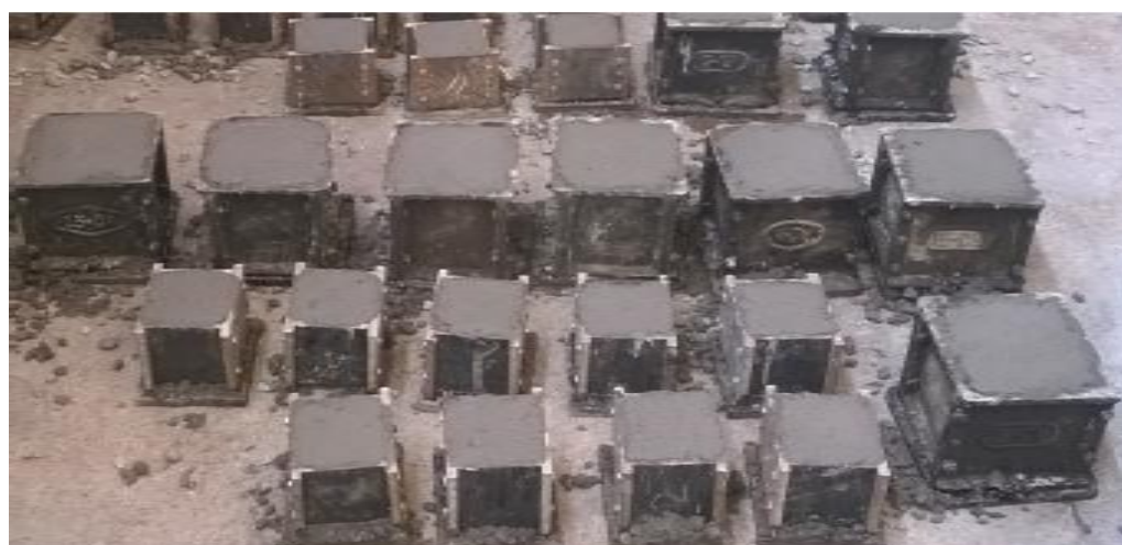
Figure 3.2: Casting of concrete cubes for compressive strength
