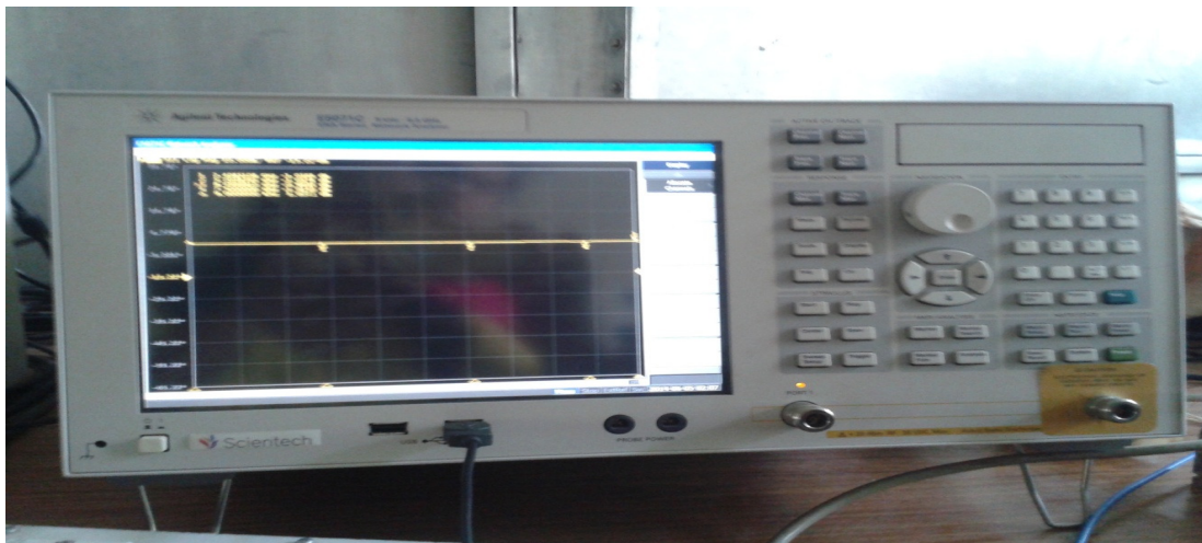
Figure. 5.10. Vector Network Analyser for testing
