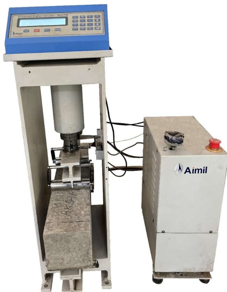
Figure 4. 10 Beam in Flexural Testing machine
