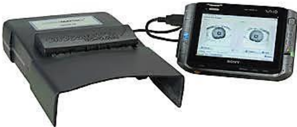
Figure 2.12: ISCAN-2 iris scanner [56]
