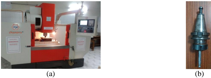
Fig. 3.1 (a) Three-axes BFW (Chandra +) CNC milling machine and (b) adapter assembly
