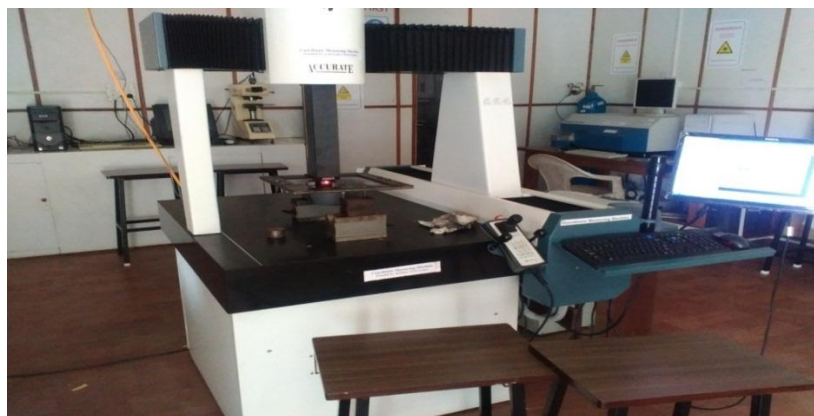
Fig. 3.12 CMM used for the reverse engineering
