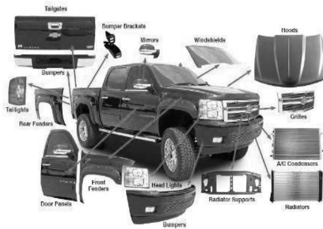
Fig. 1.2 Metal sheet parts in major panels of car body [3]
