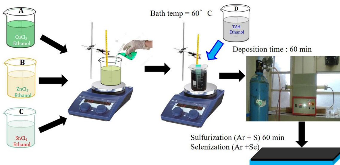
Fig. 2.2: Schematic diagram to illustrate various steps used for the deposition of CZTS(Se) thin films.
