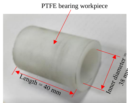
Fig. 6.18. PTFE bearing workpiece along with the dimensions.
