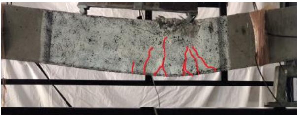
Fig. 5.10: Typical crack patterns
