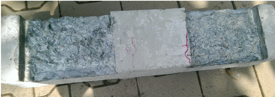
Fig. 3.9 Epoxy Layer Applied After Chipping off (Stage 2)
