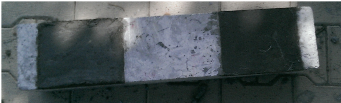
Fig. 3.10 Beam Retrofitted with UHPFRC (Stage 3)
