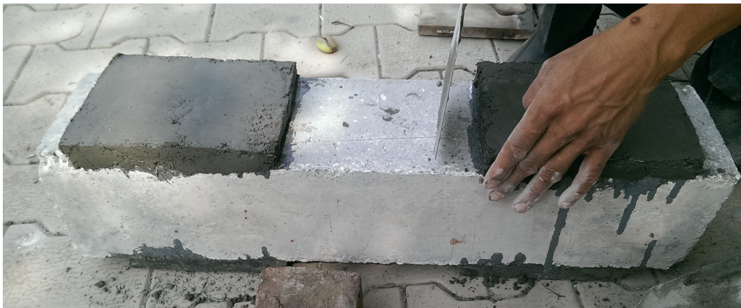
Fig. 3.12 Beam Strengthened with 25 mm Thick UHPFRC layer
