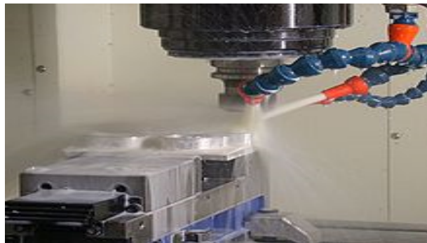
Figure1.10: Water-miscible cutting fluid application [14].
