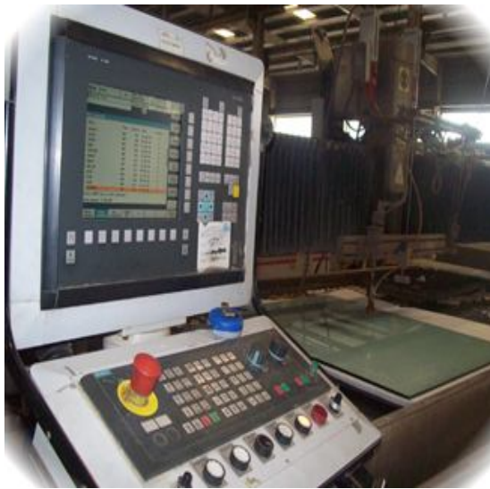
Fig. 2.13: CNC water jet machine (Courtesy: GSC GLASS Pvt. Ltd, Noida)
