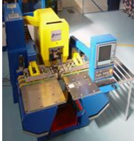
Fig. 2.9: A picture of CNC diamond drilling machine (Courtesy: Asahi India Pvt. Ltd)
