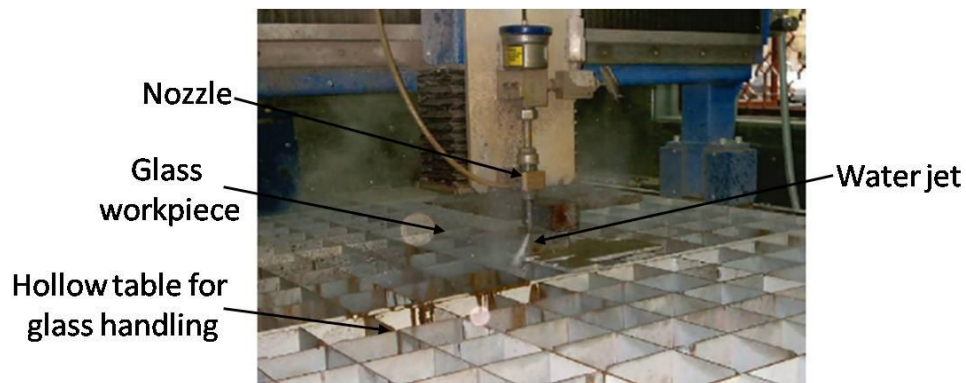
Fig. 1.6: Abrasive Water Jet Machining (AWJM) process (Khan and Haque (2007)).
