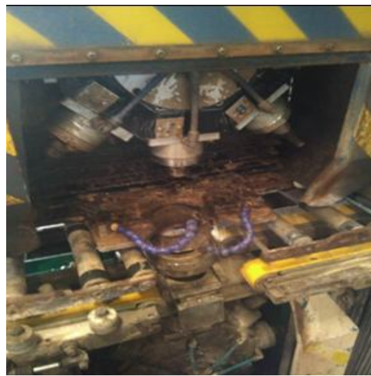
Fig. 2.14: CNC double-ended drilling machine (Courtesy: GSC GLASS Pvt. Ltd, Noida)
