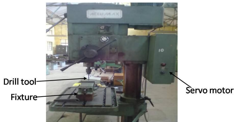
Fig. 1.5: Conventional diamond drilling machine (Navanth and Sharma (2013))
