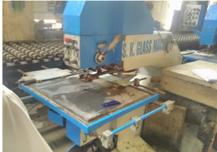
Fig. 2.15: Conventional diamond drilling machine
