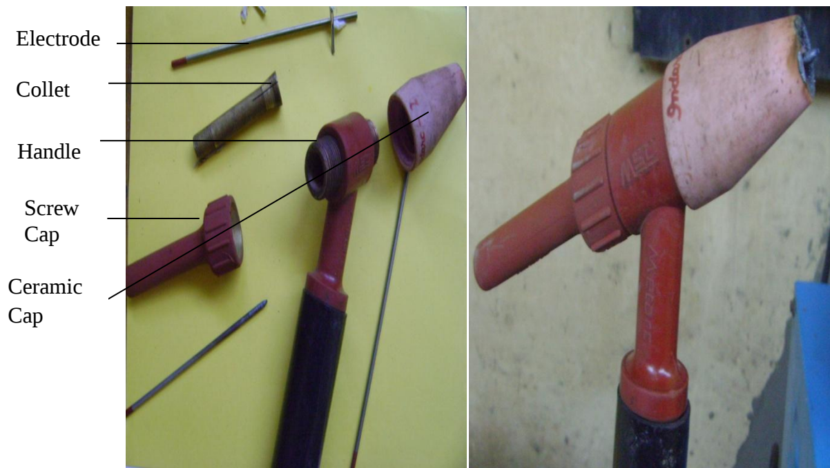
Figure 1.6: GTAW torch with handle, electrode, ceramic cap, screwed cap and collet ( Courtesy: Central Workshop, Thapar University, Patiala)
