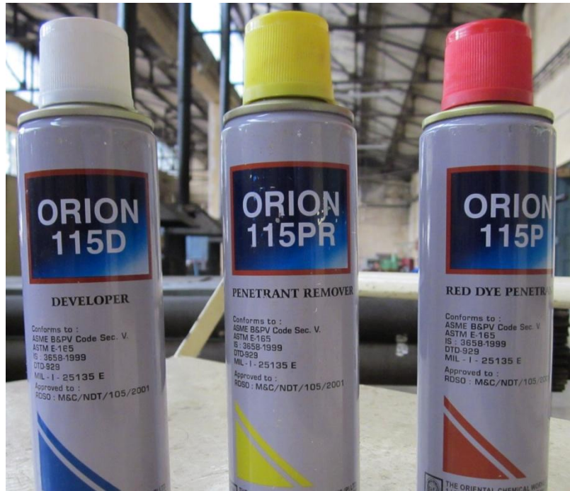
Figure3.29: Cleaner, penetrant & developer to be used for DPT test of specimen Steps while performing DPT test were as under:
