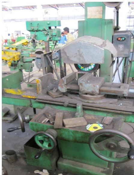
Figure 3.15: Surface grinder machine. (Courtesy: Central Workshop, Thapar University, Patiala)
