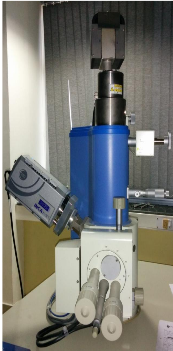
Figure 3.30: Scanning Electron Microscope (Courtesy: SAI lab, Thapar University, Patiala)
