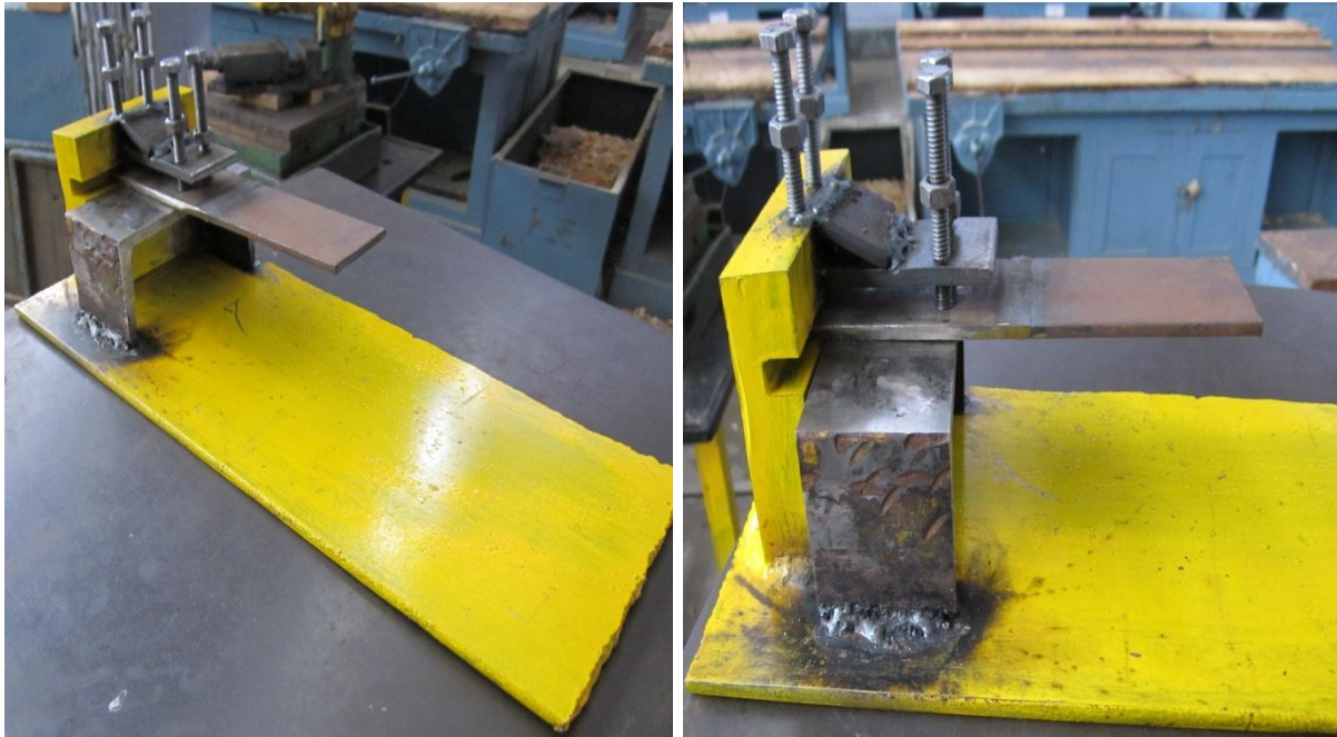
Figure 3.28: Distortion measurement by fixing the plate by screws.
