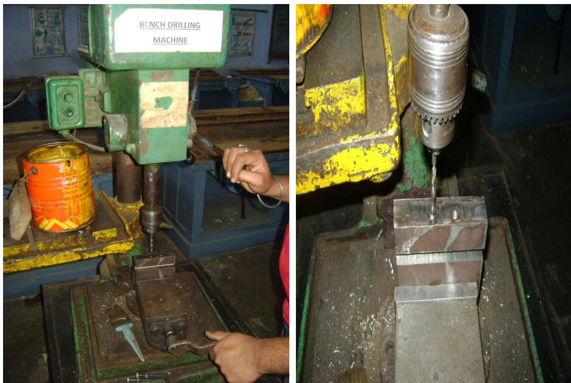
Figure 3.26: Bench drilling machine (Courtesy: Fitting shop, Thapar University, Patiala)
