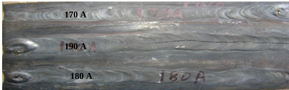
Figure 3.3: Pilot experiments at 170 A, 190 A and 180 A current on AISI 4340
