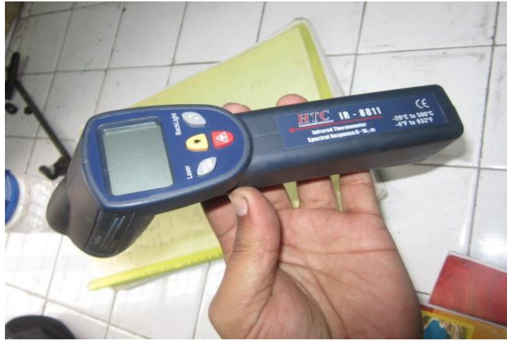
Figure 3.9: Infrared thermometer used for the measurement of temperature
