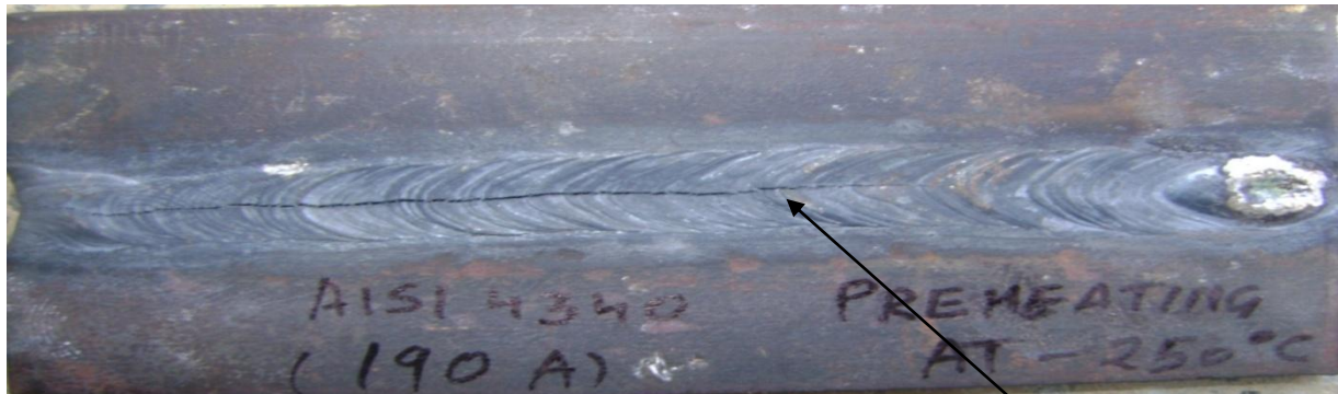
Figure 3.7: Pilot study AISI 4340 having current of 190 A and pre-heating temperature at 250 °C
