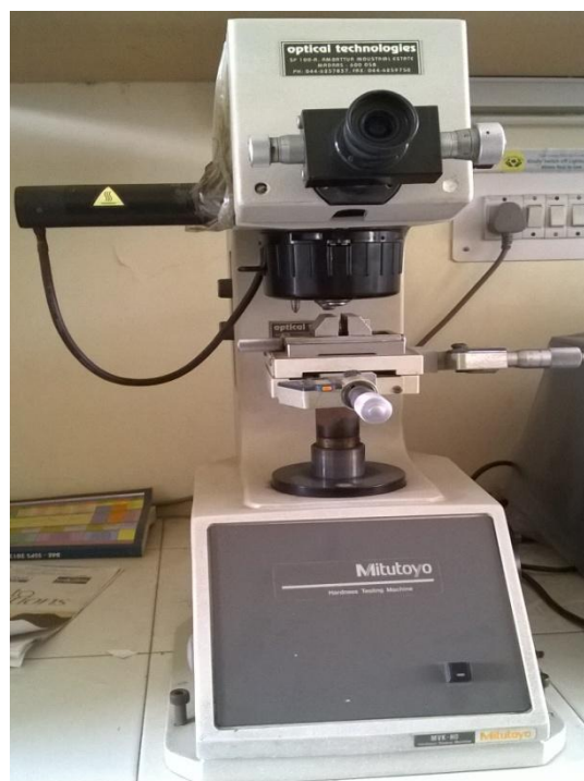
Figure 3.23: Hardness testing machine (Courtesy: Physics Department, Thapar University, Patiala)
