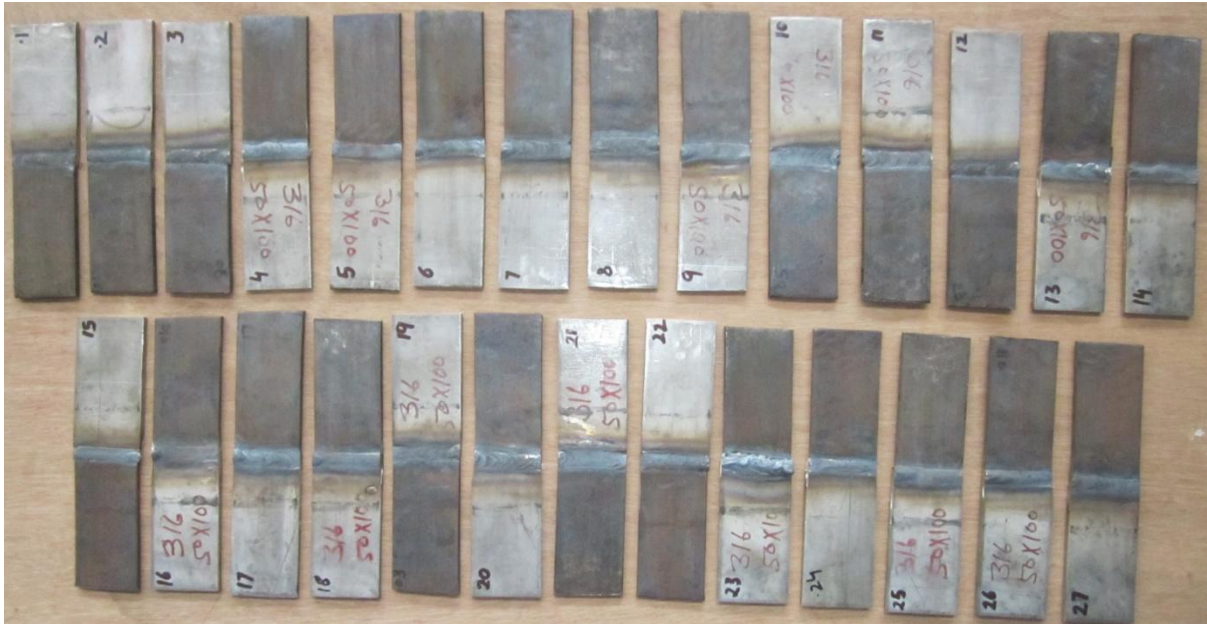
Figure 3.14: Specimens of AISI 316 welded with AISI 4340 grade stainless steel immediately after welding
