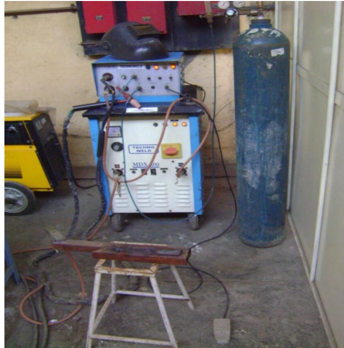
Figure 3.1: TIG welding setup ( Courtesy: Central Workshop, Thapar University, Patiala)
