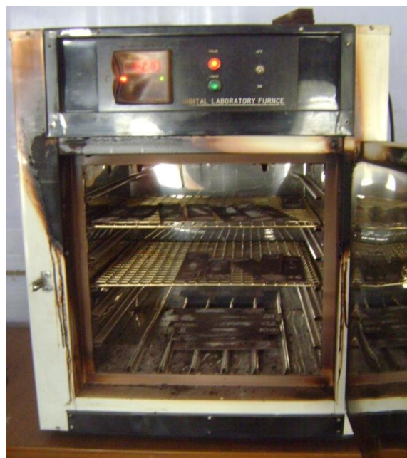
Figure 3.8: Baking oven used for pre-heating temperature.
