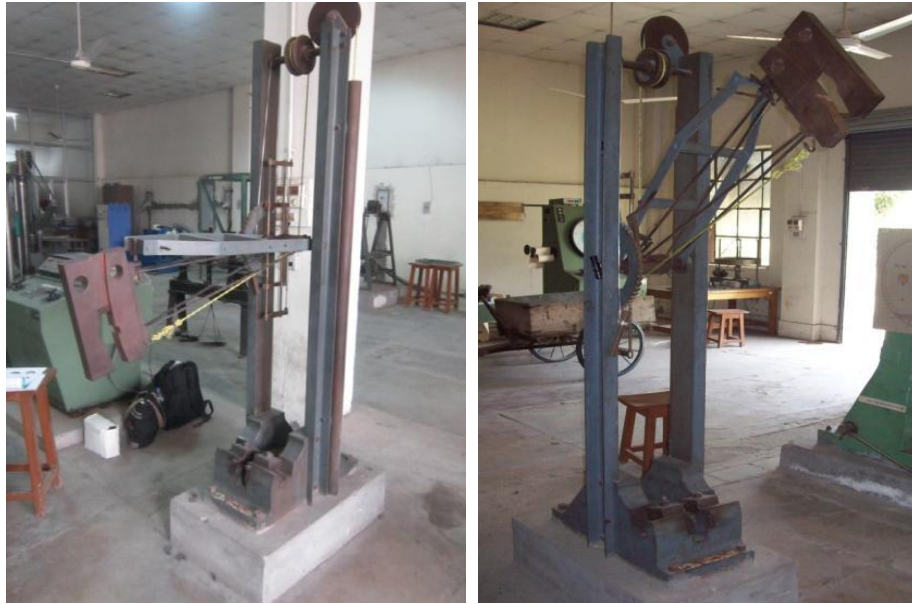
Figure 3.20: Impact testing machine (Courtesy: Solid Mechanics Lab, MED, Thapar University, Patiala)
