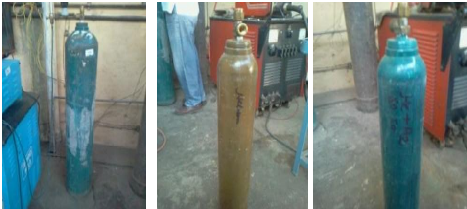
Figure 3.5: Cylinder of argon gas, 70% Ar + 30% He gas and argon - hydrogen 1.5% mixture gas
