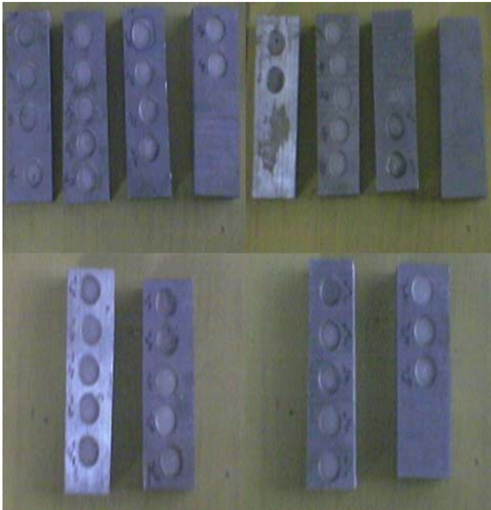
Figure 5.1: Straight polarity machined surfaces with/without addition of powders.
