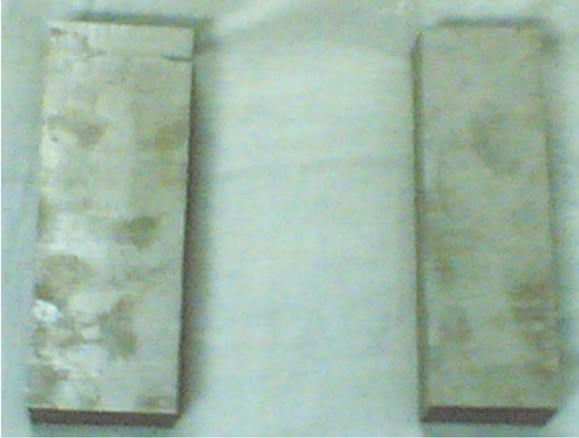
Figure 4.4: Workpiece EN 24 Steel
