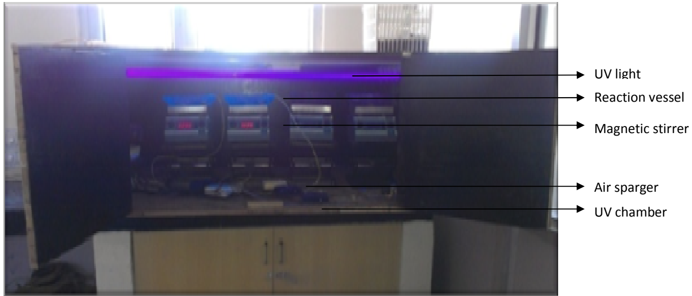
Figure 4.2 Photo reactor at lab scale during photocatalytic treatment
