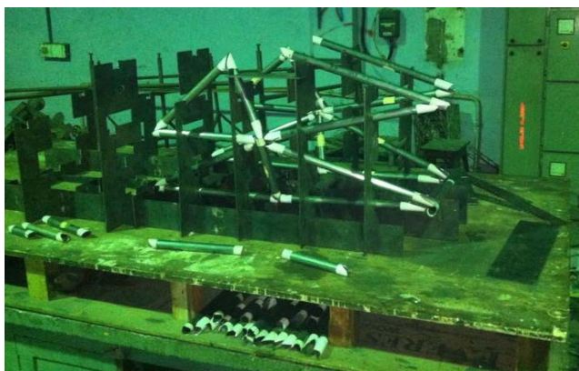
Fig 8.4: Front portion of TU FSAE 2014 Chassis supported on Jigs
