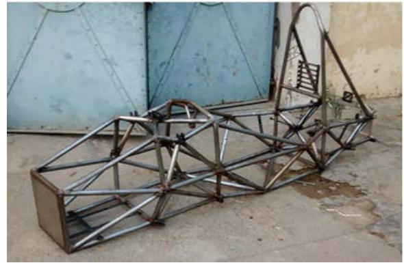
Fig 8.8: 2014 Chassis front part (completed) Fig 8.9: Final completed 2014 Chassis with Bulkhead
