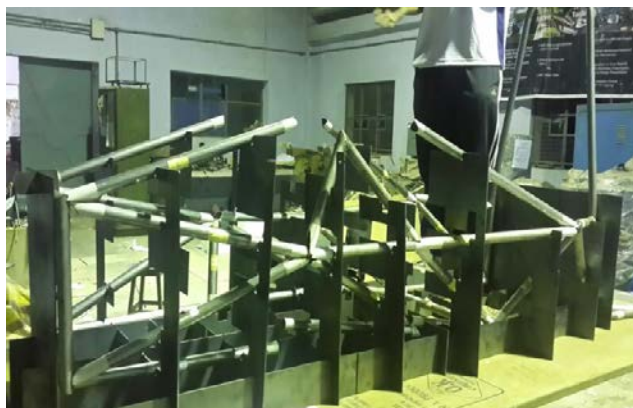
Fig 8.4: Front portion of TU FSAE 2014 Chassis supported on Jigs
