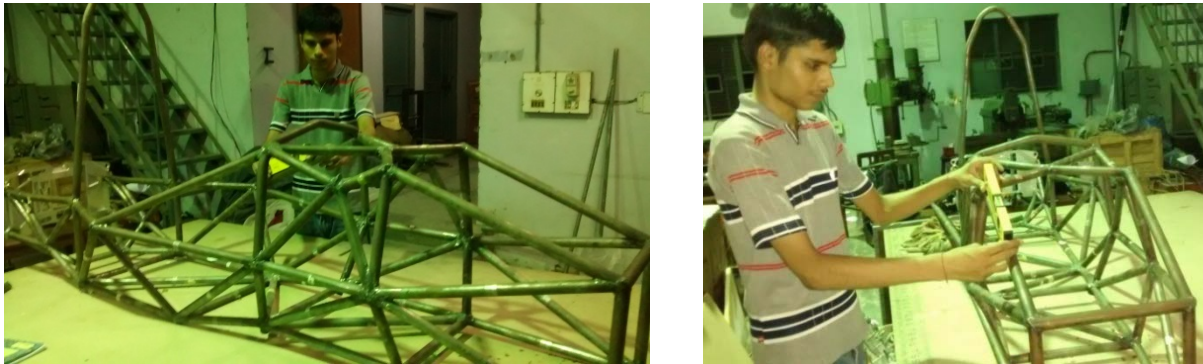
Fig 8.7: Checking process in order to verify Chassis dimensions & angles
