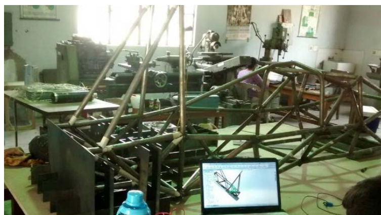
Fig 8.5: Rear portion of TU FSAE 2014 Chassis supported on Jigs
