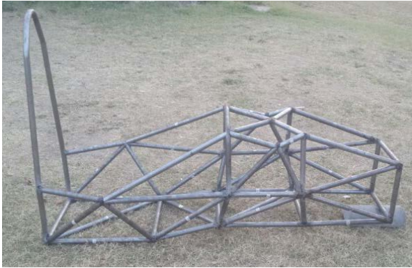
Fig 8.8: 2014 Chassis front part (completed) Fig 8.9: Final completed 2014 Chassis with Bulkhead
