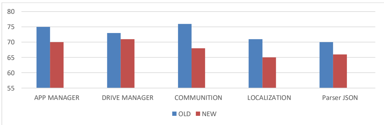
Fig.6.2. Used RAM for each WD Drive Agent application's version after various tasks execution
