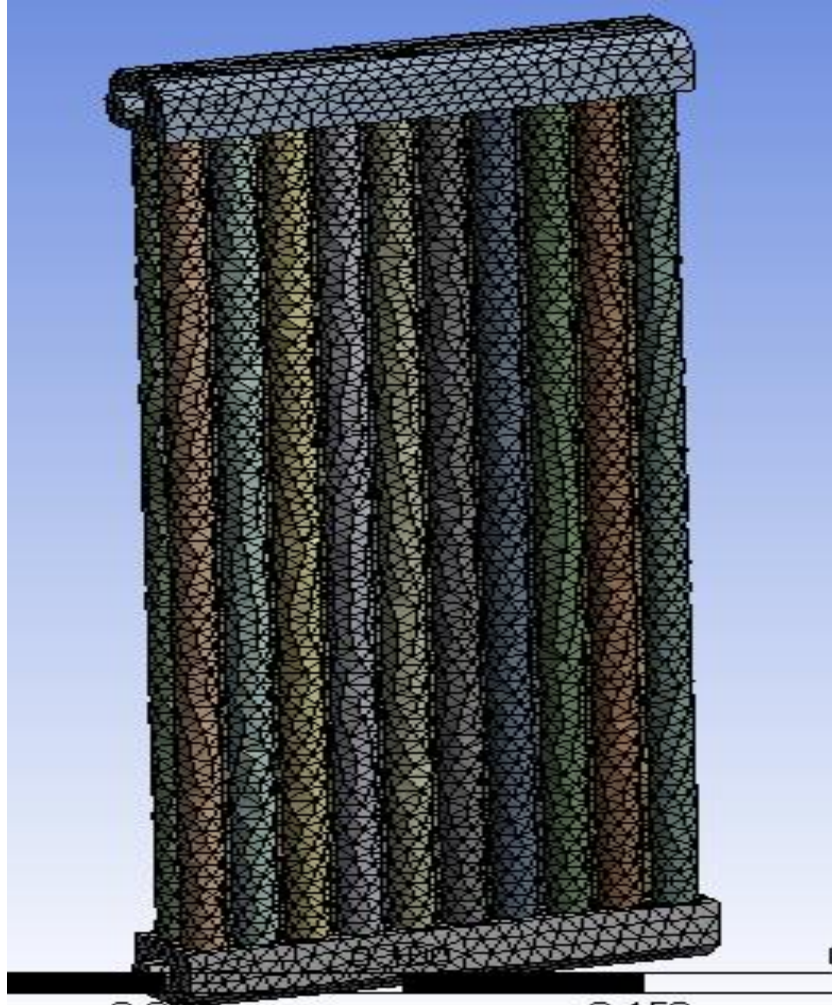
Figure 6.12: Meshing of Radiator
