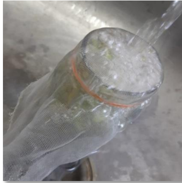
Fig 6: Washing of samples under running tap water
