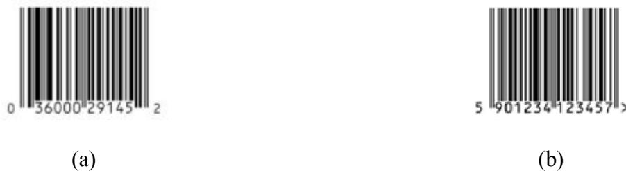
Figure 2.3 (a) Universal Product Code (UPC) - A barcode symbol. (b) European Article Number (EAN) -13 barcode symbol.
