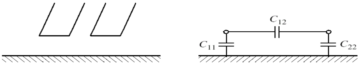
Fig. 1.3 Transmission line and Capacitive network [4]
