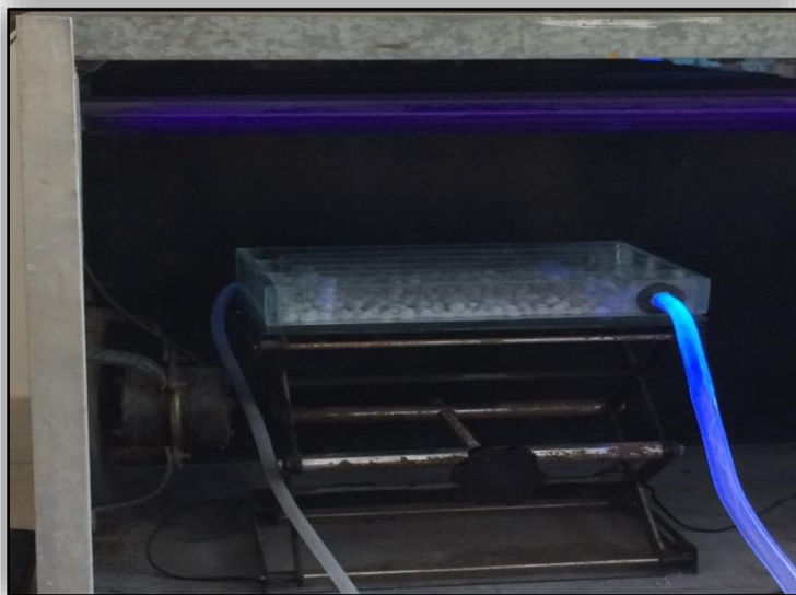
Fig 4.3: Experimental Setup consisting of UV chamber and fixed bed reactor
